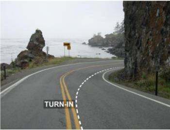
The best way to maximize the view is to enter corners from the "outside" of the turn. That is, approaching a righthander, make your turn-in from a position closer to the centerline.
