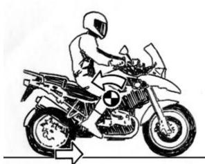
In a corner, it would be best to maintain the weight distribution on the tires. Even if the bike is in a straight line, rolling on the throttle tends to shift weight onto the rear wheel. Rolling off the throttle shifts weight toward the front. That same front-rear weight shift occurs in a corner. To maintain traction, it would be best to maintain weight distribution while leaned over.
