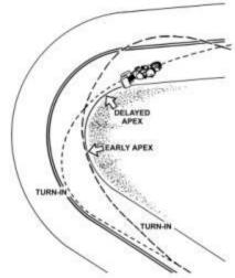
We often describe our cornering lines in terms of the "apex"-the imaginary point where the motorcycle passes closest to the inside of the curve. The location of the apex determines the shape of your line. If you turn in early and point the bike toward the inside of the curve too soon, you'll pass by an "early" apex. The problem with an early apex is that you're tempted to carry too much speed into the turn, and then halfway around, realize you're running wide.
