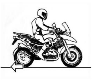
note that rolling off the throttle is also rear wheel braking, as engine compression tries to slow the rear wheel.
