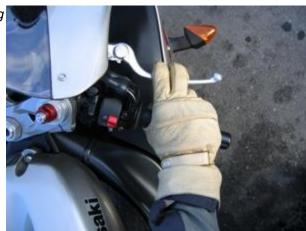
Controlling the throttle and brakes simultaneously requires some right hand dexterity. You'll have to find a technique that works for you. Some riders prefer to hold the throttle with thumb and forefinger and brake with the three outer fingers. Others prefer to hold the throttle with thumb and outer two fingers, and brake with the two inner fingers. Which fingers you use for braking may depend upon the force needed at the lever on the bike you're riding.
