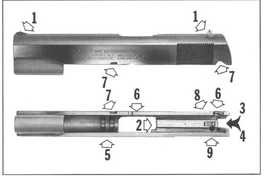
Figure 40- Shows the slide body fully cleaned, ready for final inspection. As with the frame, closely inspect and detail the areas listed below. Naturally, an excellent frame shouldn't be mated to a slide in anything less than top condition.
