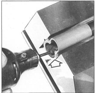
Figure 45- Shows the newly staked sight stem being ground to flush inside the slide. Use a Dremel tool and a tapered or conical grinding head. Caution: Remove just enough material to allow free movement of the barrel bushing, beyond this point, too much of the rivet may be removed, weakening the connection.
