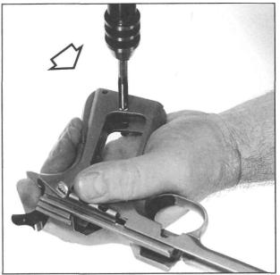
**Figure 110-** Shows re-tapping the frame to the larger 255 X 60 size to receive an oversized grip screw bushing. Generally, this is done by hand. Frames with heavy thread damage would be the exception. In these cases, a tapping guide or drill press mounted tapper should be used to prevent damage to the remaining material.
