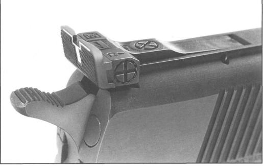
Figure L- Shows a Colt National Match Gold Cup with a Millett Series 100 Gold Cup Sight Installed. The sight fits perfectly into the factory milled slot- but I suggest that you replace the factory pin. Both windage and elevation adjust at 1/8 per click, at 25 yards. Requires a .200" front sight.
