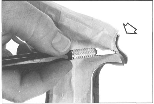
**Figure 212-** Shows the frame sides, top, and rail slot areas masked in preparation for partial sandblasting. Masking tape will not adhere unless all surfaces are clean and grease free. Remember to protect the rail slots. Trim excess masking tape away with a sharp Exacto knife. When the sides of the frame are to be sandblasted also, mask only the rail slots and top of the frame.
