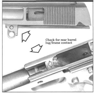
Figure 91- Shows the slide assembly completed except for the link-down check, [also called a long link check]. When longer barrel links have been used to increase engagement of the upper lugs, the back of the bottom barrel lug may contact before the barrel can fully link down to position in the frame's barrel recess, or bed.
