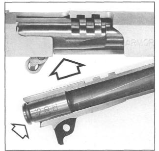
Figure 73- Shows a commercial "no-go" headspace gauge in the chamber. This gauge measures .920", which is .022" longer than "go". Barrel/slide combinations that will close and lock on this gauge have serious problems. The issue here is safety and responsibility. Don't fail to make this critical test when fitting.
