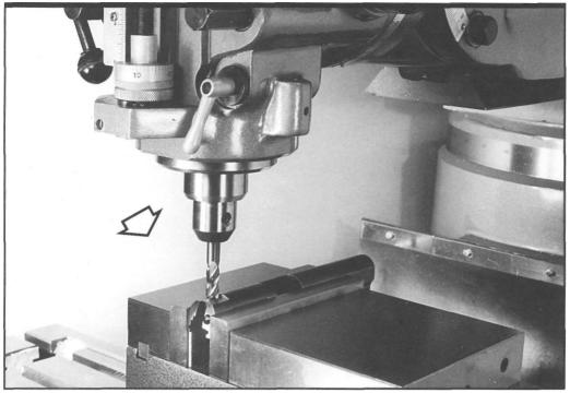
**Figure 191-** Shows the slide being milled to receive a custom low profile type sight. When this step is done, the new dovetail is located and then cut while the slide is in the same set-up position. Select the correct angle sight base cutter [either 60 or 65 degree] before milling the dovetail slot. **Caution:** Tips will break if cutters of this type are rotated at speeds beyond about 600 to 700 rpm.
