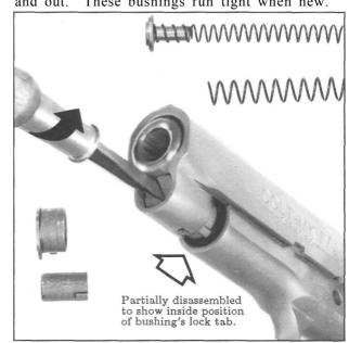
Figure 8- Shows the barrel bushing removed and the recoil spring plug pushed in and ready to rotate to its' release point at about 180 degrees, or 1/2 turn. Use caution: this short, double spring system releases abruptly. The recoil spring plug and the two special recoil springs are shown separately above.
