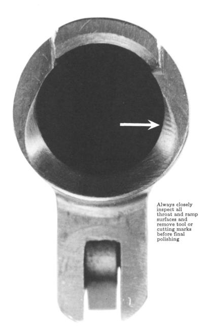
Figure AA- Shows an enlarged rear view of a Colt .45 auto barrel after rough throat and ramp contour shaping and stoning. When completed, the last step is to fine polish the newly contoured areas. This chamber entry modification assists feeding when wadcutter or other flat nosed cartridges are used.
