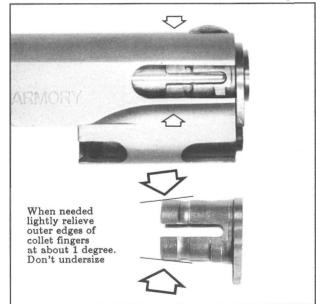
**Figure 55-** Shows a cutaway slide with bushing in view. Arrows indicate the areas inside the slide where all machining high spots should be polished and removed. Approximate bushing relief, or clearance, angles are also shown. This angle is shallow and should agree with the slide when the bushing is fully expanded.
