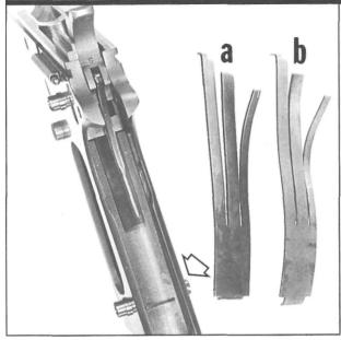
Figure 140- Shows the sear spring retaining slot machined in the frame to hold the sear spring in correct vertical position. Curvature of the standard factory sear spring is shown at "A" and a reduced power spring at "B". Standard springs measure .036" to .0375" thick. Reduced power springs are thinner, measuring .034" to .035".
