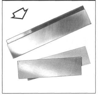
Figure 153- Shows both single and double-side rail forming and gauging bars. These hardened, surface ground bars are used as an inside frame rail forming die by holding them inside the rail slots as the rails are peened, or swaged lower. The bars are also useful as a measuring device for checking rail slot height and condition.
