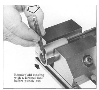
Figure 42- Shows the front sight being removed using the original punch-out method. Punching the sight out from the inside prevents exterior finish damage. Sights can be removed from the top, by the faster draw-out method, with vise grip pliers and a copper leverage block, but the potential for finish damage is much higher.
