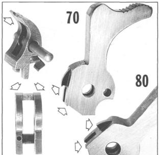
Figure 122- Shows both Series 70/80 Gold Cup hammer inspection points. Sear engagement on both runs .018-.020", but the difference is that the Series 80 no longer has a captive half-cock notch. Series 80 stop ledges average about .070" tall. The same sear is used for both models and must be inspected for engagement condition.
