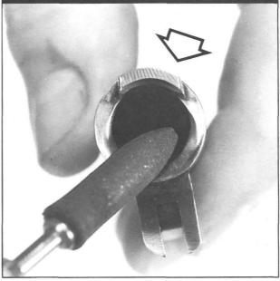
Figure 186- Shows the barrel ramp being radius polished with an extra fine, round end, Craytex tip at point "A". Only an area of about 1/4" to 5/16" of the barrel ramp is radiused, as shown. Correct tool angle is approx. 15 degrees toward the bore. At this angle, the round-off is a very slight .001" to .002". See caution at figure 187.
