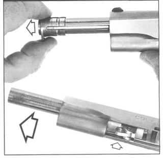
**Figure 15-** Shows the correct removal of a series 70 or 80 collet style bushing, by drawing it straight forward and off the extended barrel with your fingers. The barrel is also set up for removal from the slide. The link is shown rotated forward until it rests horizontally on the barrel in front of the bottom lug.
