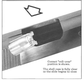
Figure 188- Shows an empty shell in the just ejected, "roll-over" position. The empty case contacts the ejector and literally rotates out of the ejection port. When a roll-over clearance notch is milled into the slide, the shell clears the port much earlier, leaving the inside port area free to cycle the next cartridge.
