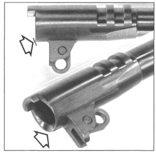
**Figure 96-** Shows the approximate barrel face dressing angle necessary when the barrel ramp must be moved slightly forward to provide clearance between barrel and frame ramps. It is not adviseable to move or clearance the entire barrel face, since the upper surface is needed when the barrel is in the locked position.
