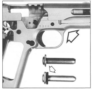
**Figure 111-** Shows a cutaway view of the front part of the frame. The slide is to the rear in the full recoil position. The back surface of the slide's spring plug housing has stopped the slide and is in full contact against the recoil spring guide's base plate. A spring guide is shown below with a shock absorbing buffer installed.
