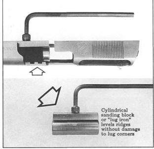
Figure 66- Shows a .650" round brass sanding and truing block, or "lug iron", being used to level the slide lug area. The theory is that machining ridges and flanging are better leveled by first truing and polishing at 90 degrees to the lugs. Thin #240 wet-dry automotive paper, followed by #320 grit, is best for this job.
