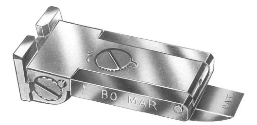
**Figure J-** Shows a large view of a **Bo-Mar** sight, similar to the **BMCS**, but on a modified base to fit Colt Gold Cups. Bo-Mar says this sight is now discontinued. What was good about this sight is that it provided a sight radius closer to 7". It's fairly easy to to make custom variations of this base on a mill and then install a BMCS in it- if your customer just has to have one for his Gold Cup.
