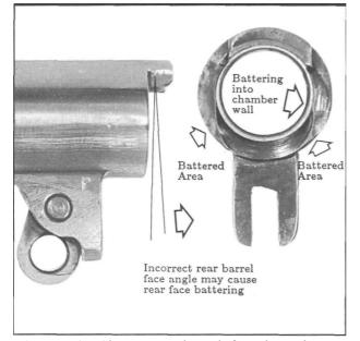
Figure 70- Shows rear barrel face battering on a standard, unthroated M1911 military barrel. When severe, the chamber mouth can be peened and damaged. Battering shown is deeper at the bottom, usually indicating an incorrect barrel face angle. However, always make sure that a high spot in the slide hasn't caused the problem.
