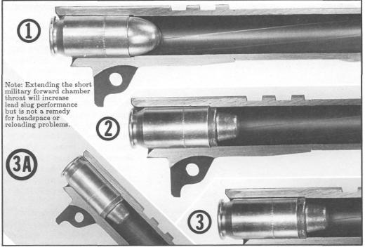
Figure 75- Shows four examples of different .45 ACP rounds chambered in half-sectioned barrels with varying amounts of headspace.
