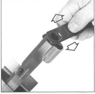
Figure 52- Shows hand seating a newly turned and dressed competition, or accuracy type, bushing. Use a steel bushing wrench for this job. Prevent finish damage to the slide and bushing by applying a protective layer of masking tape to the face of the wrench. Work in with J.B. Compound and final seat with oil.
