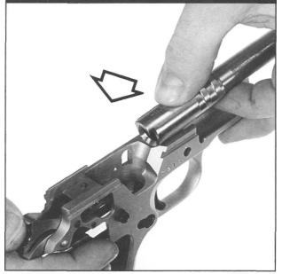
Figure 95- Shows checking the new linkeddown, full contact barrel position against the frame's barrel bed. Distance between barrel and frame ramps will have changed as a result of bottom barrel lug trimming and set-back. If necessary, adjust the rear edge of the barrel ramp back to about 1/32". See figure 96.
