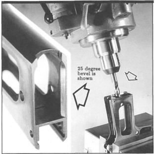
Figure 193- Shows the bottom of the frame and magazine well, after it has been bevelled. A milling angle of about 25 to 30 degrees will provide the best opening that can be machined into the thickness of the frame. If you use external add-on funneling devices, such as the Speed-E-Loader, do not mill the frame.
