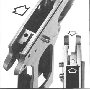
**Figure 117-** Shows inspecting the disconnector port at the top and inside of the frame. The port should be round, not oval, with an inside diameter of approximately .160". Distance from port centerline to the back of the magazine well varies with well sizing, and may not indicate a port problem unless it is less than about .195".
