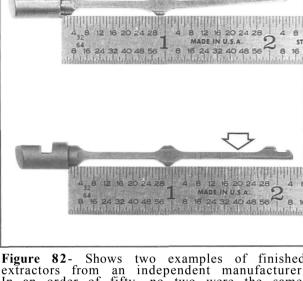
Figure 82- Shows two examples of finished extractors from an independent manufacturer. In an order of fifty, no two were the same. When ordering and replacing extractors on a one time basis, there is a tendency to install the new part "as-is", on the reasoning that, since it's a new part, it won't likely need fitting. Not so.
