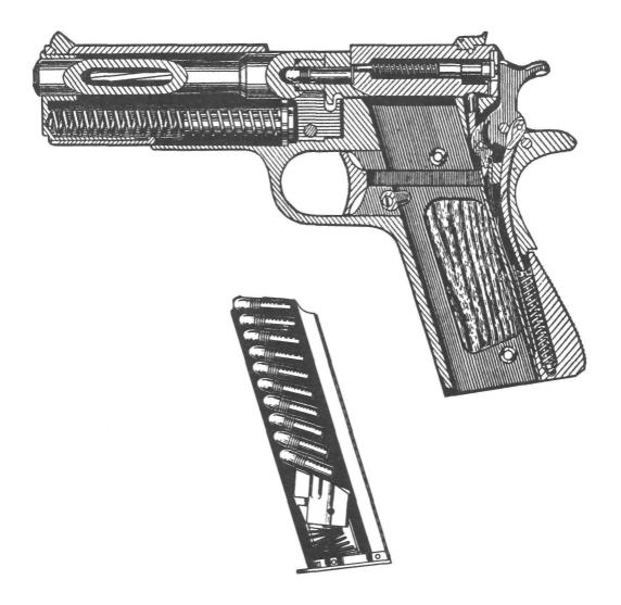
Parts Diagram Colt Ace .22 L.R. Caliber Service Model
