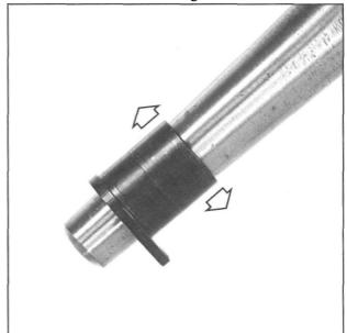
Figure 49- Shows a bushing skirt expanded on a tapered expander punch. This is the standard way to tighten bushing fit inside the slide. Reducing bushing movement improves overall accuracy in service pistols. For match use, barrel to bushing clearance also must be reduced, requiring an accuracy type bushing.
