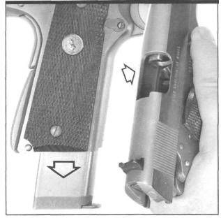
Figure 1- Shows removing the magazine and then locking the slide assembly back. Warning: always unload and clear a pistol or revolver before inspecting, handling, or doing any kind of work, whatsoever. Visually, check the chamber. Double check by inserting the tip of your little finger, if lighting is poor.
