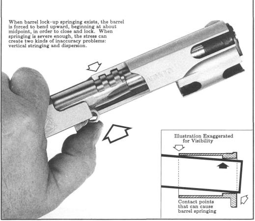
**Figure 59-** Shows the test for barrel springing, done by thumb depressing the barrel and lugs into the fully locked position in the slide. As you do this, carefully feel to determine whether or not the barrel has to be sprung [slightly bent] in order to go into full-lock. When springing is present, the barrel feels somewhat like a leaf spring. As the barrel fully locks, it should become solid in the bushing, having taken up all vertical slack and without binding or springing.
