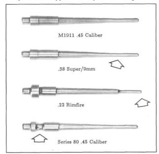
**Figure 77-** Shows examples of four basic firing pin variations, M1911, to date. You will notice that the 9mm and .38 Super firing pin has a narrower .070-.071" tip, and that the .22 Ace and .22 conversion firing pin is for rimfires. Series 80 firing pins are shorter than earlier models, and are relieved for the stop plunger.
