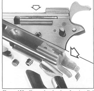
Figure 138- Shows the thumb safety installed temporarily, to check frame fit. This is done before the plungers are installed so that bind or drag can be easily detected. The dual plunger and spring assembly is also shown. Note the correct dog-leg at spring center. A doubled pipe cleaner is the best plunger tube cleaning tool.
