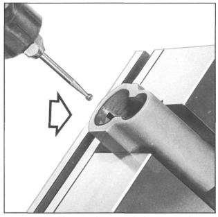
Figure 43- Shows where an indent must be cut around the sight stem passage inside the slide. A Dremel tool and a .125" round ball cutter is used for this job. Just enough material must be removed so that the soft sight stem has room to flow into the slide. The stem is then flared and riveted in place with a sight staking tool.
