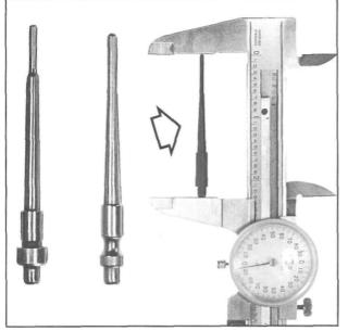
Figure 76- Shows measuring firing pin length with a dial caliper. In theory, inertial firing pins are designed shorter than their recesses, providing extra safety clearance. These firing pins must over-travel to contact the primer. Excess length may be dangerous in the event the pistol is dropped. Always check length.
