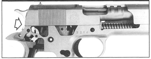
Figure 133- Shows a cutaway view exposing both the hammer and sear in an M1911A1 type pistol. With the hammer in the rest position, the sear is against the outer wall of the hammer's half-cock notch. As the slide closes, the disconnector moves up, ready to pick up the sear when the hammer is cocked.
