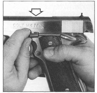
**Figure 12-** Shows proper removal of the slide stop, after aligning the stop retainer tip with the relief cut in the slide. Press the rounded end of the cross pin up from the back side, drawing the slide stop lever up and out of the frame with fingers. **Caution:** Don't pry. A drop of all usually traces a stuck slide stop plupger of oil usually frees a stuck slide stop plunger.
