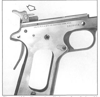
**Figure 132-** Shows installation of a Series 80 hammer/strut assembly in a Series 80 frame. This is best done with the right side of the frame up, as shown. With hammer positioned, the plunger lever is slipped sideways into place. The lever fits into the small recess milled in the right inside of the frame. See figure 130.
