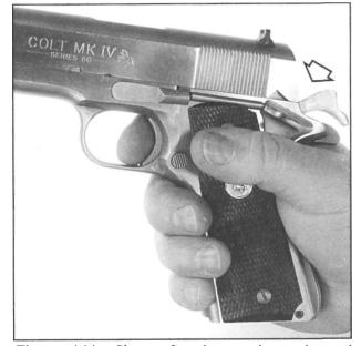
**Figure 144-** Shows function testing grip and thumb safeties; both must prevent hammer fall. After sear work, the sear's safety shoulder may be slightly forward at full cock. If shoulder clearance exists, the thumb safety stop stud may not be able to prevent sear release. In this case, sear or safety replacement may be required.
