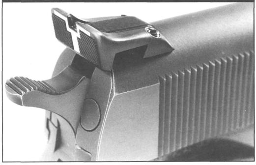
Figure N- Shows a Colt Government Model with a Millett Mark II, Low Profile Sight installed. Two set screws lock the sight in the factory dovetail. This very easily installed sight extends useful sighting radius by approximately 5/8".
