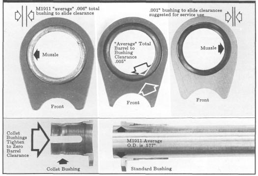
**Figure 58-** Shows "average" slide/bushing and bushing/barrel clearances in M1911 and civilian pistols. With collet type bushings, forward clearance measurement is not as important, since barrel contact is further back and inside the bushing. See inset. By this time, probably a lot more than four million M1911, A1, and civilian versions have been produced. With age, wear, and the diversity of manufacturers, a fair amount of dimensional variation can, and does, exist.
