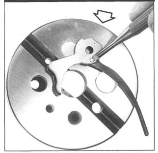
Figure 127- Shows the hammer/strut assembly positioned on a bench block, ready for staking the hammer strut pin. When the strut pin has been properly staked on both sides, and the sides of the hammer dressed, all possibility of the pin backing out and dragging inside the frame has been completely eliminated.
