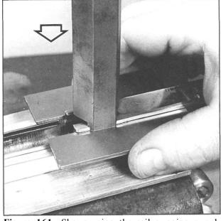
Figure 161- Shows using the rail swaging punch to lower the frame rail ends. Just as with the peening method, swaging is done in a series of controlled taps, except with a much heavier, 12 oz. hammer. It is important that the punch be held against the rail and straight up while the rail is being moved progressively downward.
