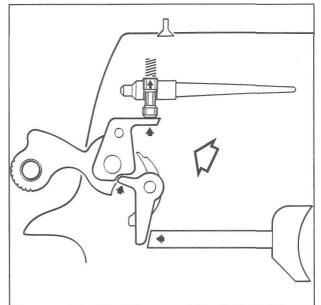
Figure 130- Shows the interaction of Series 80 safety features, as a safety reminder, and also to caution about the factory fit plunger lever. This part has three fitting variations marked 1. 2, and 3. They vary in angle and elevation, and provide critical final lift for the firing pin lock. Only the original fitting number can be used!
