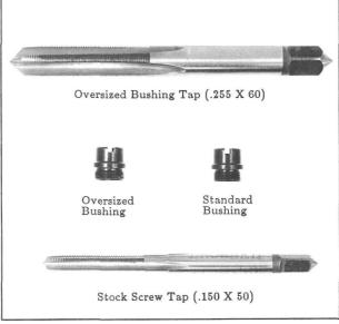
Figure 109- Shows both a standard size and an oversized grip screw bushing. [.235" O.D. threads and .254" O.D. threads.] An oversized, replacement bushing tap [.255 X 60] and a standard stock screw tap [.150 X 50] are also shown. In most cases, the .255 X 60 will re-tap stripped standard bushings without drilling.
