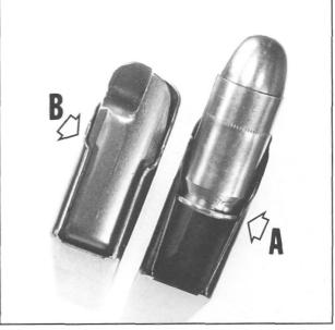
**Figure 206-** Shows the inside lip and polishing areas at "A", where tapered magazine lips are dressed and slightly opened for earlier cartridge release. "B" shows the release timing rim slots in one style of parallel-lip magazine. Polishing these slots and chamfering the bottom inside lip edges will quicken cartridge release timing.
