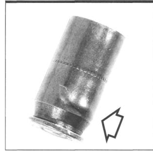
Figure 74- Shows a fired .45 ACP case with a bulged lower wall- a danger sign. This was not caused by overloading. In this example, the brass case tried to pressure form downward into an unsupportive barrel ramp area- a classic example of barrel over-ramping. Fortunately, a moderate load and high quality brass was used.
