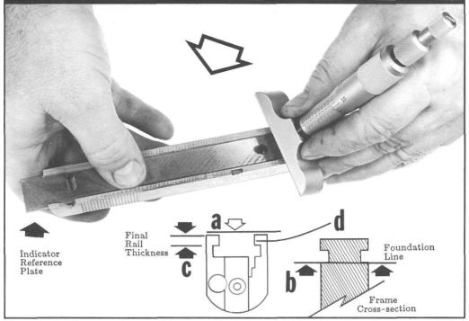
Figure 150- Shows slide measurements and checks necessary before frame rail lowering can begin. It is sometimes forgotten that the finished slide is the actual measuring reference that determines just how far the frame rails must be moved downward, or lowered.
