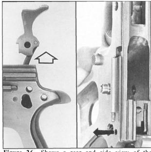
Figure 26- Shows a rear and side view of the frame and hammer. The hammer cross pin must be pushed out to the left [see arrow]. Use a small punch. This pin has a slightly beveled head, recesses into the left side of the frame, and is retained by the thumb safety lever. At left, the hammer is drawn out of the frame.
