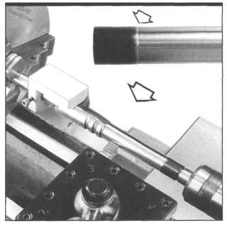
**Figure 175-** Shows a close view of the front of an oversized match barrel that has been turned to about .575" O.D. for bushing clearance. Note the necessary gradual taper where the barrel steps-up to the bushing engagement surface. Just below, a barrel is shown set up between the self aligning fixture and a live contert the self aligning fixture and a live center.
