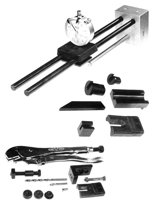
**Figure P-** Shows, at top, a very useful handgun bore sighting fixture and gauge from **Millett Sights.** The complete set includes 9mm, .38/.357, and .45 caliber barrel inserts, and measures sight height based on the centerline of the bore, which is the only accurate way. Millett's standard sight staking tool kit [single staking] is shown at center and their Dual-Crimp sight installation tooling is shown at bottom. **-Courtesy Millett Sights**
