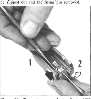
Figure 19- Shows the removal of a Series 1980 firing pin stop plate using a small punch as shown in figure 18 above. The difference is that the firing pin lock plunger [see arrow] must be depressed first in order to move the firing pin forward enough to allow the firing pin stop plate to be drawn out of the slide.
