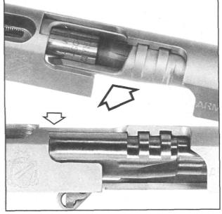
Figure 72- Shows a commercial "go" headspace gauge installed in the chamber. In the .45 ACP, headspace is measured from the case mouth back. The slide must close easily on a "go" gauge, which measures .898" in length, the same as maximum case length. On final fitting, check all replacement barrels with a "go" gauge.
