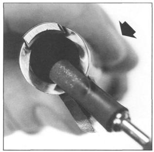
**Figure 185-** Shows the chamber throat as it is being blended-in with the barrel ramp. Then, the combined throat and ramp surfaces are fully polished. The Foredom tool is used again, this time with Craytex rubber-abrasive polishing tips. A medium tip is excellent for blending, and fine, or extra fine, for final polishing.
