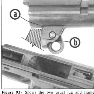
Figure 93- Shows the two usual lug and frame contact points resulting from increased link length. Since frame and barrel lug dimensions vary, there is no way to predict just what link length will produce lug contact. Sometimes, the lug/barrel radius will contact first at location "A", but usually contact will be at location "B".
