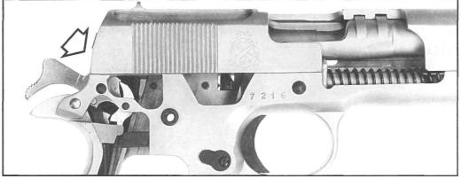
Figure 135- Shows an M1911A1 cutaway as above, with the sear now engaged in the full-cock position. In operation, as the slide closes, the disconnector is automatically cycled upward to pick up the sear hooks. Firing is possible. The thumb safety can be engaged only when the hammer is in full-cock position. The safety stop stud contacts the sear's safety ledge and prevents sear movement.
