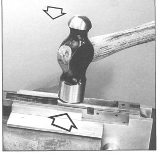
Figure 157- Shows a 6 or 8 ounce ball peen hammer positioned over the front frame rails. The hammer's face must be trued and polished to prevent excess impact marking. Only the top rail ledge 1.060" to .065"] of the frame is to be lowered. Insert the correct forming bar into the rail slots, where shown. See arrow above.
