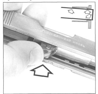
**Figure 174-** Shows the springing test, necessary after precision barrel and bushing fitting. This is a simple, yet important, check for possible inside bushing throat and skirt bind. The barrel must go into the full-lock position without the slightest bend or stress. Inside bushing bind and contact areas are also illustrated above.
