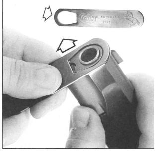
Figure 5- Shows using a bushing wrench to remove tight fitting accuracy type bushings and collet style barrel bushings. Wrench use can leave wrench marks on the face of the slide and also the bushing. There are tough plastic wrenches on the market which will, except for the tightest bushings, eliminate this problem.
