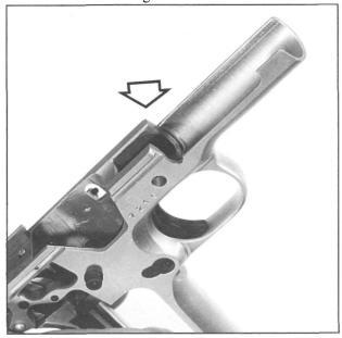
Figure 112- Shows the frame rail ends where set-back and dressing is required when the slide contacts the front of the frame rails at the same time it contacts the spring guide's base plate. These abnormal, early stops against the front edges of the frame rails batter the rails, and are an indication of mis-fitting of slide and frame.
