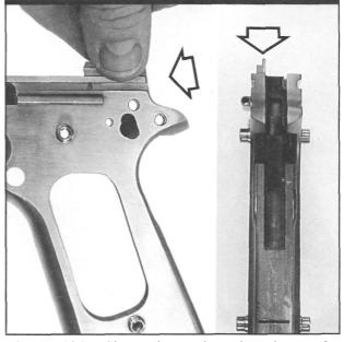
Figure 101- Shows inspecting the ejector for straightness and proper fit on the frame. The ejector body should rest squarely on top of the frame without space between it and the frame, and without side play or any detectable up or down movement. The retaining pin should be just slightly below flush on either side.
