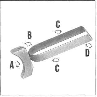
**Figure 113-** Shows four trigger check points: "A"- the trigger body should be inspected for straightness and minimum play in the frame, "B"- check for tight connection of trigger bow and body, "C"- check the bow for straightness and frame fit, "D"- inspect for correct frame position of the rear engagement surface.
