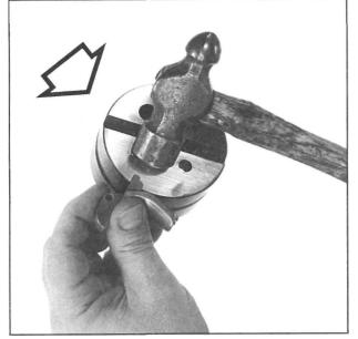
**Figure 137-** Shows the grip safety extension on a bench block, ready for stretching a slightly short tip. Use a six ounce ball peen hammer for this job. Strike the tip with a series of moderate taps until it reaches the desired length. If the stop tip requires more than .030" stretching, I suggest replacing the grip safety.
