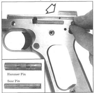
Figure 128- Shows checking hammer and sear pins before further assembly. If pin condition or fit is poor, irregular movement can cause hammer and sear positions to shift, producing variable sear releases, and, in some cases, creep. Sometimes, leaving the head of the hammer pin slightly high helps support the thumb safety.
