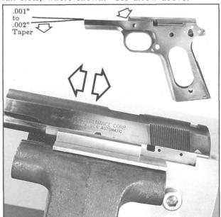
**Figure 158-** Shows trial fitting the slide on the newly tightened frame rails. It's a very good idea to make this check frequently during the lowering process. The forward portion of the frame, or recoil spring tunnel, may contact or bind, requiring extra clearance as shown above. Sometimes, gunsmiths mistake this for rail bind.
