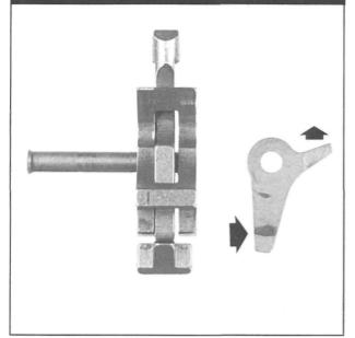
Figure 32- Shows the disconnector, sear, and trigger bar lever in a Series 80. In operation, the trigger bow actuates this lever, which, in turn, operates the plunger lever on the hammer cross pin. Both levers fit into a recess milled in the right side of the frame. This combination then unlocks the firing pin plunger.
