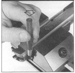
Figure 46- Shows a slide in a toolmaker's vise, secured between soft lead pads to protect the finish, ready for rear sight removal. A brass or aluminum block placed under the slide will help focus impact energy, and makes removal a lot easier. Use a brass drift for this job. Drive the sight blade out from left to right, as shown.
