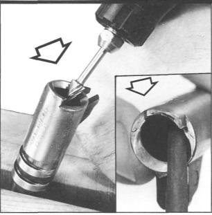
Figure 184- Shows a barrel set-up in the vise between wooden blocks to prevent tool chatter. Entry throats can be cut with a Dremel tool [at moderate speed], but a Foredom variable speed tool controls and works better, in my opinion. Some consider hand broach cutting easier. Final shaping is done with a medium India stone.
