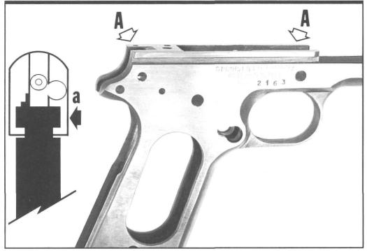
**Figure 165-** Shows an oversized National Match type frame. This frame is larger in both rail height and width, and does not require rail peening or swage-down. The two earlier systems reversed, or inverted, the bearing rails, to make the slide's bottom rails fit tightly in the frame. With this larger frame, the upper rails remain as bearing surfaces and are hand fit to minimum clearance inside the slide's original rail slots. See bearing surface indicated at "A" above.
