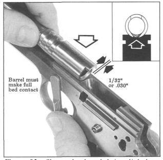
Figure 92- Shows the barrel being link-down tested in the frame. The barrel must come to rest against the top of the frame, with full bed contact. A space of about 1/32" [.030" or more] should remain between the rear position of the barrel ramp and the top front edge of the frame ramp. Slightly over 1/32" is better than less.
