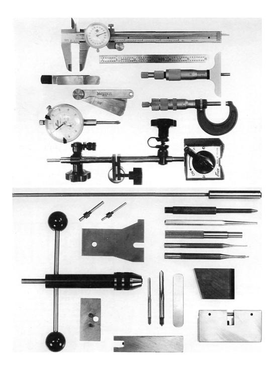
Figure V- Shows basic measuring and gunsmithing tools particularly helpful in .45 auto pistolsmithing work, including dial calipers, both inside and depth gauge micrometers, gauge stock, dies, taps, staking tools, punches, drifts, basic hammer and sear jigs, a barrel plug gauge, a thread aligning tapper and a dial indicator.
