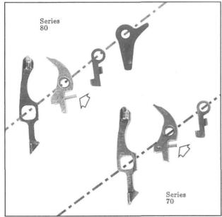
Figure 33- Shows a close view of a Series 70 and Series 80 Gold Cup sear and disconnector sub assembly. Both use the Colt Gold Cup sear, recessed for a small, extra, coil spring that acts against an additional sear depressor lever to add more sear engagement pressure, minimizing or eliminating "sear bounce" hammer releases.
