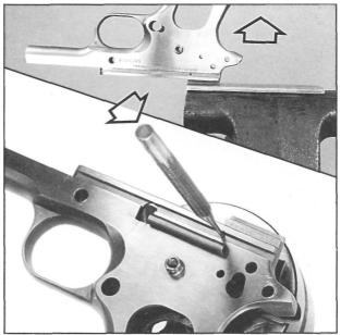
Figure 102- Shows the frame prepositioned on a bench block, set up for removal of the ejector retaining pin. The pin is punched out from left to right. Just above, the ejector is shown secured between soft brass vise jaws. Now the frame is ready to be carefully lifted straight up and off the ejector's mounting studs.
