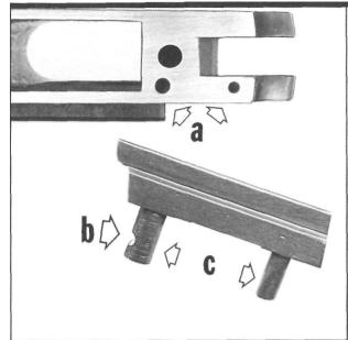
Figure 103- Shows the three frame and ejector areas which must be pre-fit before installing a new or repaired ejector: "A" shows the frame's ejector stud tunnels which require cleaning and deburring; "B" shows the ejector retaining pin notch; and at "C", the mounting studs are shown. Both studs require trimming to length.
