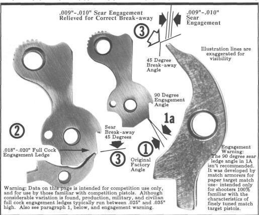
Figure 195- Shows ideal competition sear face and hammer engagement angles and dimensions. Sear escape angles and engagement measurements are also given. Competition modifications are not suggested for general or service duty use.
