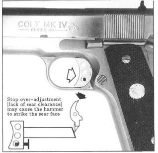
Figure 143- Shows the slide assembly and grips now installed on the frame. Below, the possible sear damaging effect of improper trigger stop screw adjustment [adjustable triggers only] is illustrated. Shorter sears finish with wider faces. Without a sear escape angle clearance cut, the risk of sear edge damage is increased.
