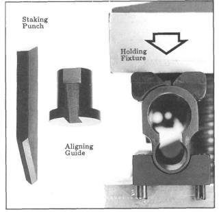
Figure 211- Shows a very workable single-stem front sight staking system, also available from Millett Sights. This tooling is designed for use in a bench vise and provides full, positive slide control, during sight installation. Correct alignment of the sight is maintained while the sight stem is being staked in position.
