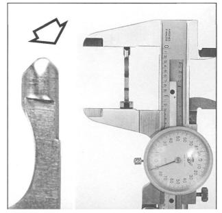
Figure 118- Shows inspecting and measuring a factory finished disconnector from a new Colt civilian model pistol. Most Colt factory fit disconnectors I have measured run 1.28?" to 1.290" overall length. Unfinished replacement disconnectors, as built by the various parts manufacturers, can exceed 1.310" in length.
