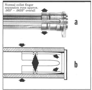
Figure 54- "A" shows normal collet diameter expansion, which results when the bushing's finger contact pads are cammed or ramped up by the bevelled back edge of the barrel as it changes O.D. "B" shows the reversed fulcrum effect created when the slide's inside clearance is too small. This stresses and bows the fingers.
