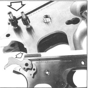
Figure 126- Shows the final mating check done on test pins installed on the exterior of the frame. Coat the surfaces with Dykem blue and hand work together. This test will show slight variations in frame pin location and alignment. If needed, minor adjustments can be made to better mate the hammer and sear surfaces.
