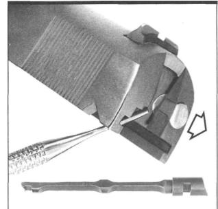
Figure 20- Shows, at bottom, the original Colt M1911 type extractor as used in all models up to and including the 1970 series. Also, an extractor head is shown in place in the slide, ready for removal. Usually, extractors are easily removed by inserting the tip of a small punch into their head slots, and pulling straight out.
