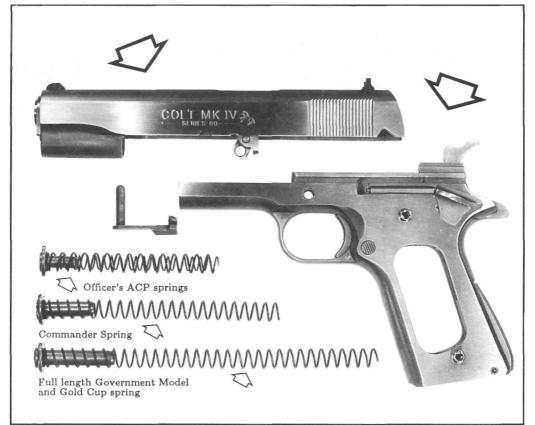
**Figure 142**- Shows the pre-fit and already finished slide assembly and slide stop, at the top. Below, the completed frame assembly is shown, except for installation of the grips which we always leave until last. At bottom, the three basic types of recoil springs are shown: standard Government Model, Commander type, and the short, double spring system used in the Officer's Model.
