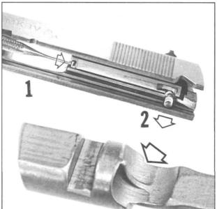
Figure 23- Shows a view of the plunger retainer stud machined into a Series 80 extractor. When the extractor is in the installed position, the plunger retainer stud is forward, keeping the plunger captive. When the extractor is moved slightly back, the retainer stud disengages, allowing the plunger and spring to be removed.
