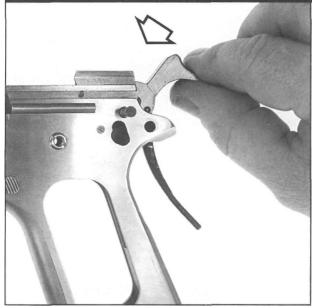
Figure 131- Shows installing an M1911 through Series 70 hammer and strut assembly in the frame. Be certain the strut pin has been staked and that drag marks have been removed from the body of the hammer. Slide/hammer side drag can be eliminated by reducing thickness of the portion of the hammer above frame level.
