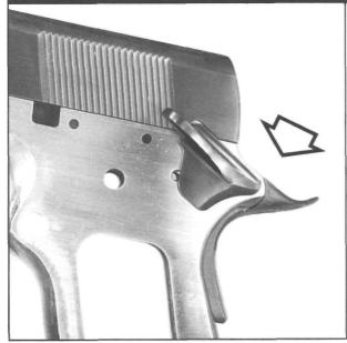
Figure 198- Shows the frame tail modified to receive a beavertail grip safety. This work is best done on a mill, using a cutting fixture, but, with care, can be done by hand. The first shaping cut should be made slightly oversized to allow for minor, individual differences in grip safeties. A hammer pin can be used for fitting.
