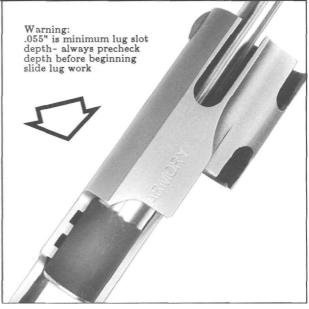
Figure 171- Shows a cutaway view of the slide with a hone being used to dress the top lug area inside. After leveling honing prepares the slide for match barrel installation and for later barrel link-up into full lug engagement. A shallow honing angle permits an increase in rear barrel elevation. Do not lower lugs below .055" depth.
