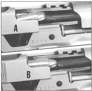
Figure 146- Shows a cutaway frame view of the dummy cartridge ramping and feeding test. "A" shows a ball round just at release from the magazine lips. At "B", the cartridge is now free of the magazine and has passed the pivot point. The rim has cammed up, into position inside the extractor's hook, as the slide closes.
