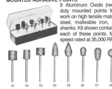
9 Aluminum Oxide (red) heavy duty mounted points for rough work on high tensile materials like steel, malleable iron, etc. 1/8" shanks. Kit shown contains one of each of these points. Maximum speed rated at 35,000 RPM.
