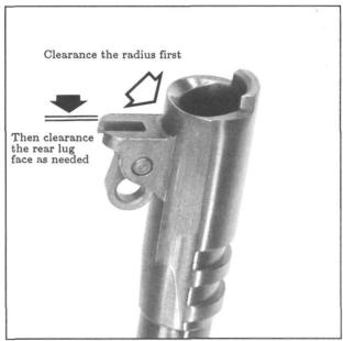
**Figure 94-** Shows the two bottom barrel lug dressing areas. In cases where the lug/barrel radius makes contact with the frame first, be sure that the leading edge of the frame's barrel bed has been 45 degree chamfered, then square the radius for additional clearance. Otherwise, slightly reduce the back bottom lug surface.
