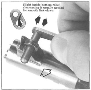
Figure 181- Shows using the slide stop crosspin, with correct link, to locate high spots or bind areas on the new lug surfaces. Remember that most lug cutters leave the lugs slightly high for final hand fitting. A 1/4" round stone is best for this work. Dykem blue will help pinpoint any remaining high spots and drag areas.
