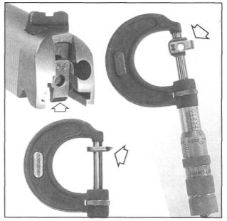
Figure 79- Shows reference measuring a loose firing pin stop plate, after checking its' fit in the slide. Finding tab size, overall plate width, and thickness, is useful in fitting replacement stops. It's wise to keep a good supply of firing pin stops on hand [currently three part numbers listed] since they vary considerably in size.
