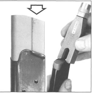
**Figure 207**- Shows tooling for closing tapered or parallel magazine lips to adjust their release points. It is also useful for complete reforming of the lips. The mandrel we received was .017" larger than the inside of any clip we have ever seen, and off in one other aspect, but such a great idea that we decided to remanufacture it.
