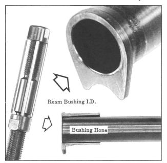
Figure 170- Shows an accuracy bushing that has been turned and sized to the slide, ready for inside barrel fitting. Adjustable reamers are helpful in pre-sizing bushing I.D. For use in competition it's important that the bushing is reamed and then honed to a light drag fit before lock-unlock clearancing and work-in.
