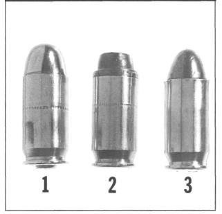
Figure 208- Shows examples of three classic ammunition problems: 1. Improperly seated primers. 2. Crushed and expanded soft lead semi-wadcutters. 3. Overly expanded and/or poorly crimped case mouths. All will affect accuracy, cause mechanical feeding problems, and are made worse by incorrect seating length.
