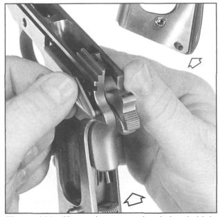
Figure 141- Shows the sear spring being held in proper position by the mainspring housing as the grip safety is slipped into place under the cocked hammer. Next, the thumb safety is put in, retaining the grip safety. Then, the hammer is de-cocked, the mainspring housing is pushed up, [capturing the safety tab] and pinned.
