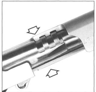
Figure 176- Shows a cutaway view of barrel lug and slide engagement. As a rule, the lug slots in the slide run slightly deeper than the height of the barrel lugs. So, the slide is dressed to allow greater vertical barrel lug engagement. Now, when locked, the rear of the barrel is tipped up a few thousandths more than before.
