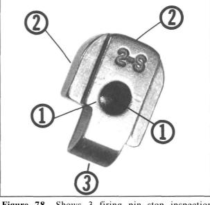
Figure 78- Shows 3 firing pin stop inspection areas. 1. Look for plate cracks, indenting, or alteration of the firing pin port. 2. Examine both back and edges for peening, punch marks, or other inexpert attempts at tightening the stop. 3. Make sure the bottom is not undersized, and is even with the slide's disconnector rail.
