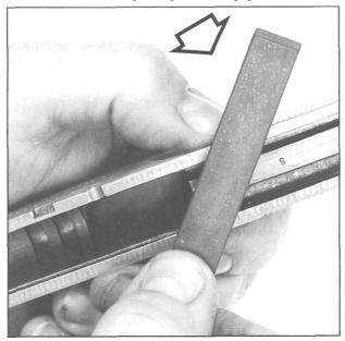
Figure 152- Shows finishing a slide bottom by hand, using a 1/2"x1/2"x6" fine cut stone. Many slides will require no more than moderate leveling and dressing with this type of stone. But some will be found with irregularities that require truing by file. Harder civilian slides should be milled as shown in figure 151.
