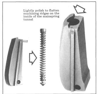
Figure 139- Shows the mainspring housing in various stages of assembly. Burrs and ridges in the mainspring tunnel can cause spring drag. Cutting the mainspring beyond two turns is not productive in reducing spring energy. A much better method is to replace the spring with a full length, but lower energy, spring.
