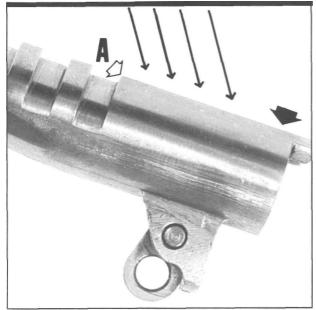
Figure 173- Shows rear barrel areas requiring pre-polishing before further fitting. The object is to provide clearance and to eliminate barrel top irregularities by cross-hatch sanding at 45 degrees. The lug tops are kept level, but the barrel top and hood are clearanced on a slight angle. The lug wall at "A" is not lowered.
