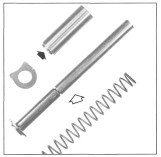
Figure 203- Shows a full-length replacement recoil spring guide. The spring plug has been drilled and clearanced for the longer spring guide stem. This system, when used with a recoil shock buffer and with the correct weight recoil spring, makes slide cycling much more consistent. Available in blue and stainless steel.
