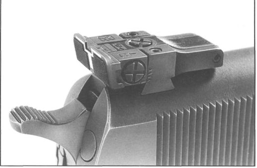
Figure M- Shows a Colt Government Model with a Millett Series 100 High Profile, Adjustable Sight installed. The high profile sight fits the standard factory dovetail, without machining, but fitting is required. A .312" front sight blade must be installed, for correct elevation.
