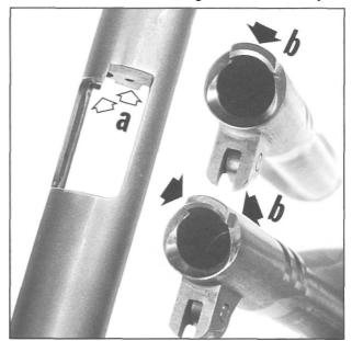
Figure 172- Shows the fitting points on a match or competition grade barrel. Match barrel hoods are oversized for precise rear barrel to slide adjustment. The arrows at "B" show where the barrel fits into the corresponding slide areas at "A". All hood edges are fit to a light drag contact, then the corners are relieved.
