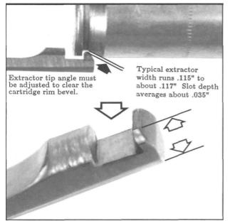
**Figure 84-** Shows the correct relief angle at the front of the extractor hook. The tip must not apply pressure inside the shell recess- correctly, tension is exerted on the rim by the extractor slot wall. Most finished extractors will measure .115" to .117" as shown above, with average slot depth at about .035" deeper than the hook tip.
