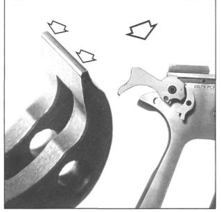
Figure 196- Shows final checking the sear and hammer engagement on external test pins before installation. After coating with Dykem Blue, mating is checked by hand operating the parts. When contact at both of the hammer's sear engagement ledges is identicad the parts are mated. The sear battering zone is also shown.
