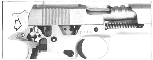
Figure 134- Shows an M1911A1 cutaway as above. The sear is now in the captive half-cock detent. With the slide still closed, the disconnector stays up and in contact with the sear. If the slide is moved slightly to the rear, the disconnector rail cycles the disconnector downward and clear of the sear's hooks.
