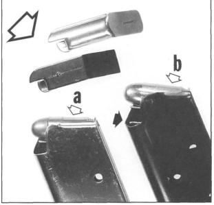
Figure 204- Shows round top and flat magazine followers, above. When control lips are not malformed or too wide at the front, round tops are generally better. The magazines below have round top followers. Both cartridge and stop tab positions are correct at "A", but overly wide lips at "B" allow cartridge and follower tip-up.
