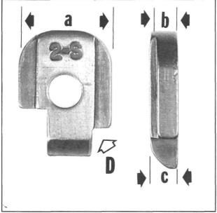
Figure 80- Shows differences in Series 80 firing pin stop plates. Series 80 stops [stamped 1 and 2] will retrofit previous models, but have the added plunger lever clearance notch at "D". Firing pin stop #1 is widest at **a**, **b**, and **c** dimensions. Stop #2 is closer in size to the original #50219 used through the Series 70's.
