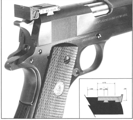
**Figure 190-** Shows a close-up view of a Bo-Mar Deluxe BMCS sight, installed on a Colt Series 70 Government Model pistol. With minor fitting, this sight fits the standard factory dovetail. Sometimes, depending on factory dovetail depth, a small clearance flat", usually .005" to .010" deep, must be milled at the top of the slide to accommodate the BMCS sight body. Once sight body position has been established, the slide is then drilled and tapped for the elevation screw.
