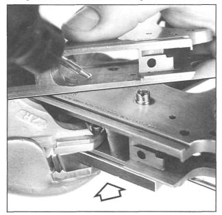
**Figure 108-** Shows the frame being prepared for plunger tube replacement. The staking holes in the frame are slightly countersunk on the inside with an 1/8" ball cutter. This extra recess helps prevent loosening of the mounting studs, once they are staked. Below, the plunger tube is shown as it is being staked in position.
