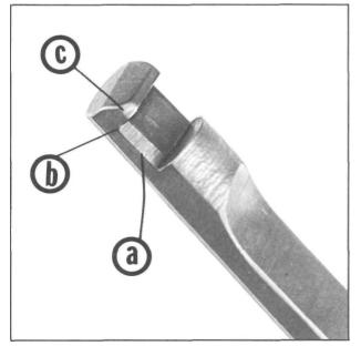
Figure 85- Shows the three bottom extractor areas requiring fitting and polishing. Cartridge pick-up is made easier by adding a 45 degree camming, or ramping, surface at slot position "A". And forward relief at "B" helps start rims into the slot, while relief at "C" provides empty shell tip-up and rim clearance during ejection.
