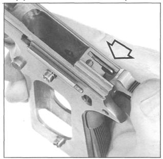
Figure 25- Shows easing the hammer forward to unload and de-tension the main spring, after the thumb safety has been removed. Caution: Never allow the hammer to strike the thin area of the frame just in front of the hammer. Strikes peen damage the frame and raise a metal edge that may interfere with slide movement.
