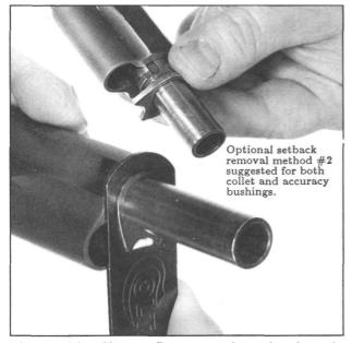
Figure 14- Shows finger turning the barreltight series 70 and 80 barrel bushings to release position after the slide has been removed and barrel set to intermediate position. The wrench removal method is shown applied to slide-tight accuracy type bushings. Bushing twist-out in this unstressed fashion eliminates friction wear.
