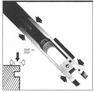
**Figure 155-** Shows the four rail end areas that are lowered when the modified rail peen-down method is used. Only a top rail area equal to the frame's slot depth should be lowered. Most rail slots run between .060" and .065" deep. Trying to peen down a wider area of the frame may damage the frame or work harden the rails.
