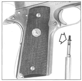
Figure 2- Shows typical wide slot, military type grip screws used in .45 autos. Always use a screwdriver that is properly ground to fit these oversized slots. To prevent grip panel damage, stone dress the edges of the screwdriver until it is slightly undersized. Disfigured screws are an outward sign of poor craftsmanship.
