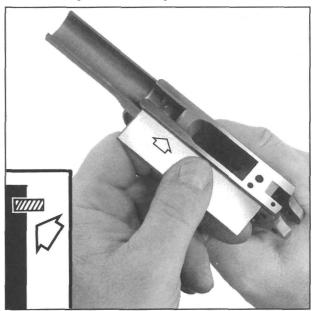
Figure 154- Shows a single-side rail forming and gauging bar inserted into the frame's ran slot, placed just as it would be when the rails are lowered. Gauge bars should be pre-selected at a size approx. .001" over actual needed slide rail height. While developing a "feel" for this work, use bars .002" over as a first step.
