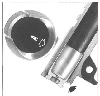
Figure 187- Shows the ramp after polishing. The cutaway correctly shows less than .090" of the brass case exposed ahead of the extractor bevel with the shell head against the recoil face, as during firing. **Caution:** More than .090" brass exposure may be unsafe- when "A" is any further forward, clearance is already excessive.
