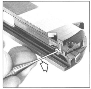
Figure 22- Shows the Series 80 firing pin locking plunger, the only outwardly visible slide difference between Series 80's and older Colt models. This spring loaded plunger serves as an automatic firing pin block. Trigger actuated frame linkage depresses the plunger, unlocking the firing pin just before hammer drop.
