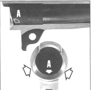
Figure 183- Shows the parts of the rear barrel face that are widened in throating. This barrel ramp widening was developed to solve feeding problems with unjacketed and wadcutter type ammunition, and also works very well with ball rounds. The location of point "A", shown above, is critical, and should not be altered.
