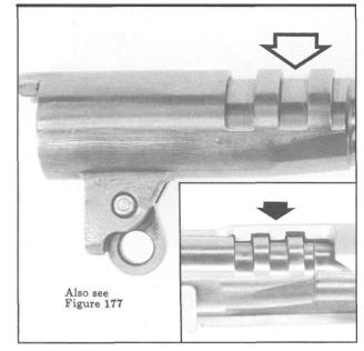
Figure 68- Shows the fast way to approximate and check barrel/slide lug engagement. 1/8" dia. strips of modeling clay are pressed into the lug slots, and compressed to final level by the barrel as it links-up. Measure lug tops down to clay level with a small depth gauge, or caliper bottom. Talc or graphite helps prevent sticking.
