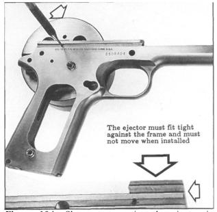
**Figure 104-** Shows test seating the ejector in the frame to make sure the mounting studs fit and that the body rests completely against the frame. The retaining pin notch must align with its' hole in the frame. Above, the left side of the frame is on the bench block as the ejector retaining pin is driven in from right to left.
