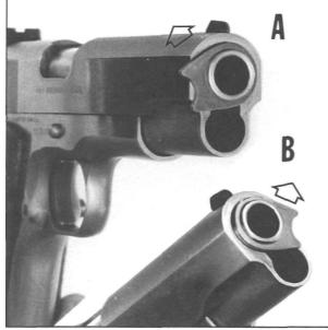
**Figure 9-** Shows barrel bushing disassembly positions for all M1911 through series 80 models. The only variation is the Colt Officer's Model, shown earlier. A clockwise 1/4 turn to the position shown in "A", above, releases the recoil spring plug, and an 1/8th turn, counter-clockwise from center, unlocks the bushing.
