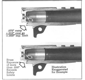
Figure 99- Shows brass exposure limits based on the formula of "go" plus .015" additional headspace when the slide and barrel are fully locked. If normal ramp exposure is .075" and headspace is "go" +.015", by this system, the amount of shell case exposed in front of the extractor bevel would be a maximum of .090".
