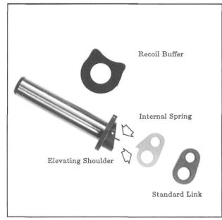
**Figure 202-** Shows a Dwyer Group Gripper and link. A standard link is shown for comparison. This simple, yet workable device contains a stiff spring which loads the shoulder of the Dwyer link. In turn, this holds the barrel at the upward limit of the link. These non-fit parts replace the standard link and spring guide.
