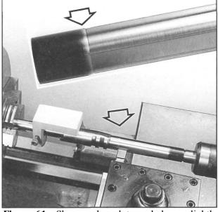
**Figure 61-** Shows a barrel turned down slightly to provide bushing skirt cycling clearance. Typical dimensions are given in the column at right. To prevent catching, the lower surface of the barrel must taper upward as it rejoins the original front diameter. Lathe set-up uses a barrel aligning fixture and a live center.
