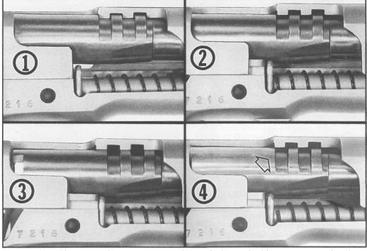
Figure 63- Shows a close cut-away view of the unlocking sequence in three normal steps, plus a fourth, where lug drag is present during unlocking. Being able to see the full unlocking sequence in a cut-away pistol is an invaluable shop training aid. The steps shown above are described in number sequence below:
