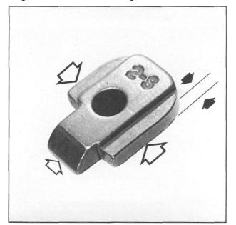
**Figure 81-** Shows the points requiring fitting or dressing when the stop plate selected for replacement is too tight. In these cases, coat the entire plate with Dykem Blue and carefully stone and clearance visible contact areas, a little at a time. Polish to a light contact fit and do not drive or force into position.
