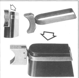
**Figure 114-** Shows the trigger bow installed on a trigger bow forming die, used with a plastic hammer in reforming damaged corners and also to straighten the sides of the trigger bow. A crooked trigger body can be hand straightened by using the die as an aligning reference. This work eliminates trigger drag in the frame.
