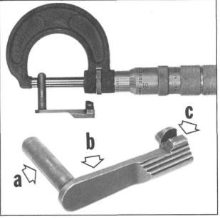
Figure 89- Shows measuring the diameter of the slide stop crosspin at the link bearing point. Below, slide stop inspection points are shown: "A" shows the link wear point at the center of the crosspin, "B" shows where to look for bend resulting from attempts to pry off the stop, and "C" shows the slide stop engagement corner.
