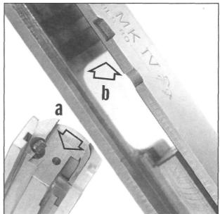
Figure 87- Shows two additional areas that sometimes require dressing and that should be checked before the slide assembly is considered complete. Check for raised edges or burrs at location "A" and slide stop flanging at "B". In the event that flanging exists, the slide stop must be checked before final assembly.
