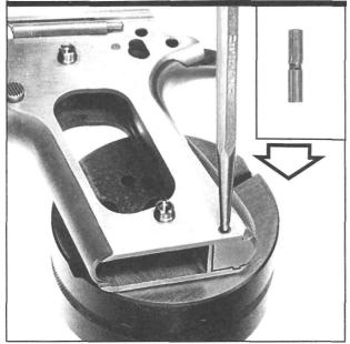
Figure 28- Shows the frame positioned on a bench block, and ready for removal of the main spring housing pin. Select a punch with tip sized small enough to fit the dimple in the cross pin. The main spring housing pin is held inside the frame by downward pressure of the pin retaining plunger, at bottom of the mainspring.
