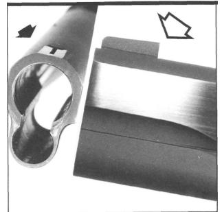
Figure 210- Shows a Millett skirted front sight in staking position on the slide. Note the small level area milled to receive the flat bottom of the skirt. When correctly installed, this sight is stronger than other single-staked types. Bonding is further increased by applying fiberglass resin to the skirt and stem just before final staking.
