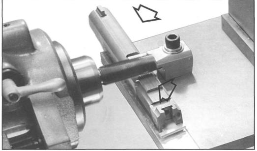
Figure 191A- Shows vee shaped serrations being milled into the top of a slide with mandrel mounted, stacked, miniature double-angle wheel cutters. For light, occasional work, this system is quite workable on a vertical mill when secure mounting fixtures are used. Carbide cutters are required for harder civilian slides; feed slowly, and use plenty of lubricant. For production work, use a horizontal mill.
