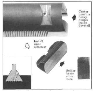
Figure 47- Shows several ways to elevate and tignten a loose rear sight blade in cases where it is important to retain the original or standard sight, and when a tighter, original style sight blade is not available. Otherwise, it is much faster and easier to replace it with an accessory type sight that has gib locks or Allen set screws.
