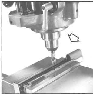
Figure 151- Shows using a carbide end mill to adjust and true the edge level of a hard, or more than slightly irregular, slide bottom after first indicating position. This method is very useful when surface irregularity is found where the recoil spring plug housing extends from the slide. Make multiple light cutting passes.
