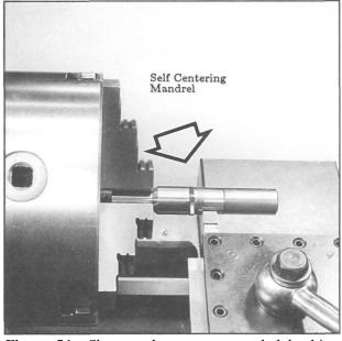
Figure 51- Shows a larger or expanded bushing set up on a self centering mandrel and chucked in the lathe. Alignment is checked with a dial indicator. In this way, the skirt is kept round and on center. Always use the rule of halves when reducing diameter: remove only half of the estimated amount, and then recheck fit.
