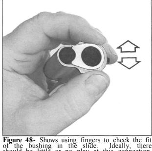
**Figure 48-** Shows using fingers to check the fit of the bushing in the slide. Ideally, there should be little or no play at this connection. Keep in mind that a variation of .001" at the muzzle equals 1" at 100 yards, or 1/2" at 50 yards. Much of accuracy is determined by how well the barrel and bushing fit in the slide.
