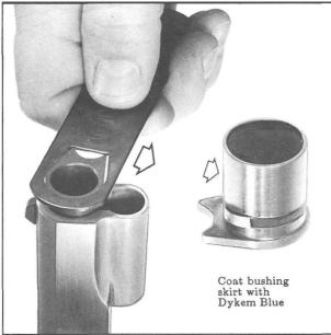
Figure 50- Shows the hand adjustment method for fitting tighter or expanded bushings to an individual slide. Binding high spots are stoned and rechecked until the desired clearance is reached. Use Dykem Blue on the bushing skirt to detect high or bind spots while trial and error fitting to the inside of the slide.
