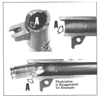
Figure 100- Shows the chamber mouth with its' sharp inside corner removed at "A" to provide "break-over" clearance for easier cartridge chambering. Break-over is the precise point at which the cartridge straightens in the chamber. Also, the inside barrel hood is shown chamfered at 45 degrees for cartridge pick-up clearance.
