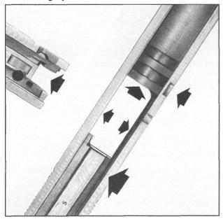
Figure 37- Shows a view of the inside of the slide and locking lugs. Since locking lug engagement is only about 60% or 70% in the average .45 auto, the lug recesses can be heavily impacted with dried oil residue, dirt, and carbon, and must be detail cleaned. Clean all other recesses; a toothbrush does a fine job.
