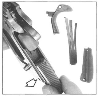
Figure 29- Shows the main spring housing being removed by drawing downward and out of the frame. Part way down the main spring housing clears and releases the bottom tab of the grip safety. Then, the sear spring is disengaged as the housing passes the bottom of the spring and its' frame retaining slot.
