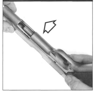
Figure 13- Shows the correct upside down way to remove the slide assembly from the frame. Get into this habit because it will prevent loss of spring guides [followers], guide buffers, etc. You may find that some pistols will have undersized and unstaked link pins which may fall out causing the loss of the link and pin.
