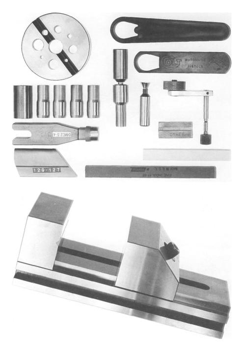
**Figure W-** Shows additional useful pistolsmithing items including a steel bench block, both steel and plastic bushing wrenches, bushing expanders, bushing turning mandrel, dovetail cutter, assorted stones, a lug cutter, sight block, and magazine tuning/adjusting tools. Shown below is a toolmaker's vise; very handy for holding and fitting small parts. I suggest buying better quality tools; they work better and last longer.
