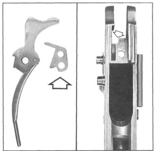
**Figure 27-** Shows a close view of a Series 80 Government Model hammer and firing pin plunger lever. The lever rides inside a slot milled in the right side of the frame and on the hammer's retaining cross pin. This slot is the only visible difference between Series 80 and earlier frames. Make sure the lever isn't lost.
