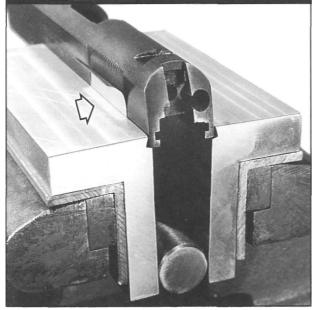
Figure 163- Shows the slide between reinforced aluminum tightening jaws. Only about 3 1/4" of the jaws bear on the slide. Shims in the finger grooves make compression more uniform. For less flex, use a large, heavy duty vise. With other variables controlled, the heavier the vise, the more predictable the final product.
