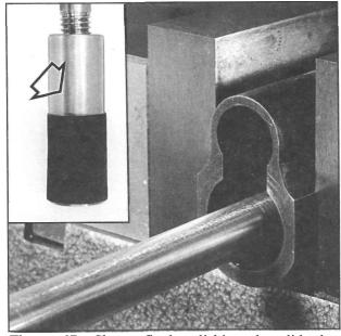
**Figure 67-** Shows final polishing the slide lug area with a rotary sandcloth hone. Use #400 sandcloth and feather the area, beginning with the ejection port, forward to about mid slide. Elevate the hone very slightly as shown. Don't lower the surface by more than .002" during the combined truing and polishing operations.
