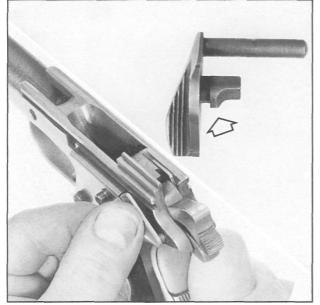
Figure 24- Shows the hammer pre-positioned at full-cock. This is the first step in removing the thumb safety from the frame. The thumb safety is held in the frame by engagement of its' shoulder recess [see arrow] and the frame wall. When in the forward position the hammer body prevents movement of the safety.
