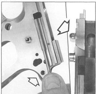
Figure 106- Shows checking the plunger tube for proper position and tightness against the frame. Also, an insert gauge made from an old 7/64", or comparable wire gauge size, drill shank is shown being used to check the larger I.D. bore portion of the plunger tube. Check the smaller front diameter with an .089" drill shank.
