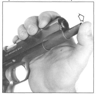
**Figure 4-** Shows decompressing a Government Model recoil spring and releasing its' stored energy. Use your thumb for this job. Springs can vary from a standard Government Model 16 lbs. up to 24 lbs. for maximum hard ball loads. Similar loads in Combat Commander pistols may require spring weights up to 26 lbs.
