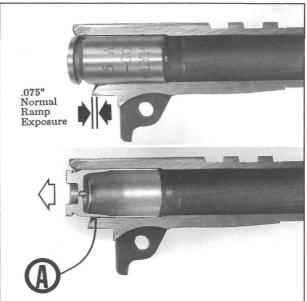
Figure 98- Shows bottom shell case exposure increased as it would be under firing pressure. The case head is pushed back against the recoil face, adding to the .075" normal ramp exposure just ahead of the extractor bevel in the case. Caution: Cartridge case exposure begins at point "A", which makes this location critical.
