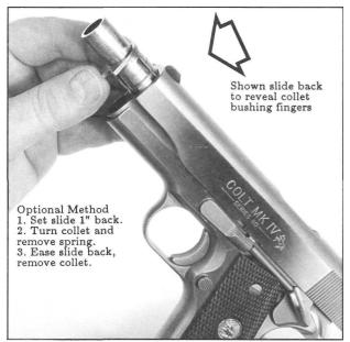
Figure 6- Shows the optional slide set-back disassembly method. The theory is that friction is eliminated between both barrel and collet by holding the slide back approximately 1" to relieve tension before turning. To improve view of the collet, the recoil spring and plug have been taken out. Also see Option 2, Fig. 14.
