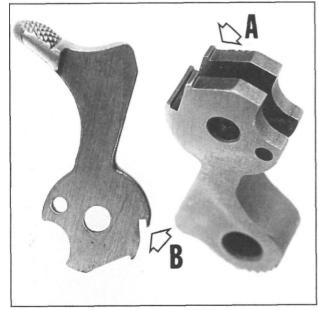
Figure 120- Shows the two hammer inspection areas important at this time since the hammer and sear are mated parts. "A" shows a close view of the sear engagement notch, measuring about .025" to .035" deep on the average hammer. "B" shows the half-cock notch, made captive in all models until Series 80 production.
