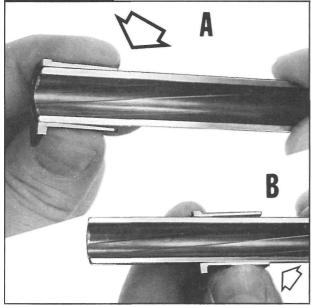
Figure 60- "A" shows a possible bushing/barrel inside bind area found when larger diameter replacement barrels and tightened bushings are used. And "B" shows the bottom contact, or drag, area which is usually present when top contact is found. Bind or friction must be removed by clearancing the barrel and bushing.
