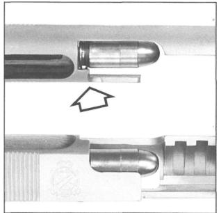
Figure 83- Shows a top and side cutaway view of a ball round being held in the slide by about 3 1/2 to 4 1/2 lbs. of extractor pressure on the cartridge rim. Without enough rim pressure, or tension, extraction can be erratic. And, with an excess amount, the rim can't cam upward into proper position without friction or hesitation.
