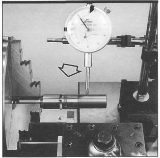
Figure 169- Shows a larger, or accuracy type barrel bushing set up on a lathe mandrel. Some oversized bushings are ribbed and/or otherwise irregular on the outside, making direct dial indication difficult. To prevent lathe tool tip breakage, use H.S. steel tooling for this work insteadof carbide. Set the lathe at low rpm.
