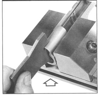
Figure 44- Shows the slide pre-positioned inside the vise, with a blade alignment block underneath. The sight staking tool is also shown in the correct flaring position, with the mouth opening clearing the slide. Caution: Do not overstrike. The sight stem must be slowly expanded until it fills the ground-in recess.
