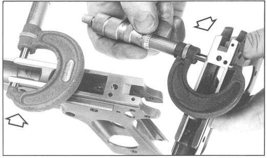
**Figure 166-** Shows measuring dimensions of the oversized N.M. frame rails for final adjustment. Both height and width must be reduced by stoning- or, preferably, by use of **a** surface plate. Fit rail height and width, and then dress until the slide will just fit onto the frame. At this point, the slide should drag evenly on the rails. Carefully remove sharp corners, burrs, and etc. from both slide and frame. Use oil when checking fit. Do not force or gall.
