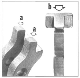
Figure 197- Shows two areas where light, final polishing is needed when precision competition trigger work is done. At "A" the sear hooks are shown, which require light, by-pass polishing. And, at "B", the sear spring engagement bevel at the bottom of the disconnector is polished. Both make disconnector cycling much smoother.
