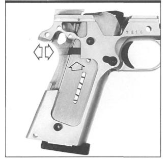
Figure 115- Shows a cutaway view of the frame exposing the trigger bow. The magazine and bow are shown being clearance checked in their normal positions inside the frame. The trigger bow is checked for magazine contact. The trigger body should be reinspected for drag as it is moved back and forth in the frame.
