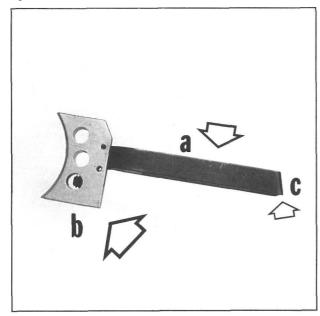
Figure 194- Shows points on adjustable, custom triggers that require inspection and/or fitting. The bow "A" and trigger body "B" both require fitting to the frame. See figures 113 through 115. The bottom rear edge "C" of the trigger bow is a sometimes overlooked area that can cause disconnector problems when left too long.
