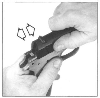
Figure 164- Shows final seating a tightened slide on a modified rail frame. When correctly compressed, the slide will finish just to a light drag fit. Drag is removed by lapping with JB bore, compound. Lap with oil and 3F silicon carbide powder to remove heavier resistance. After cleaning, hand seat the slide with oil.
