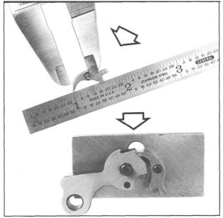
Figure 123- Shows, at top, the quick reference system for pre-checking minimum sear size. A fitter's test block is also shown being used to inspect correctness of sear angle and amount of engagement. With correct engagement and sear angle, and surfaces in well polished condition, further fitting work is not usually needed.
