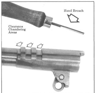
Figure 65- Shows lug areas requiring clearance chamfering when slide disconnect timing causes excess drag, flanging, or corner hits. Warning: Don't remove any more than about 10% of lug height, or a maximum of .005", with most lugs. Depending on actual lug engagement, even this small amount may require a longer link.
