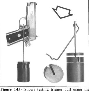
Figure 145- Shows testing trigger pull using the military/NRA type weight system. This method is simpler and more consistent than the average spring scale. Unlike sprung devices, weights can be helpful: for example, a light tap usually releases the sear when you are about a 1/4 lb. from the mark, making tuning much easier.
