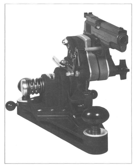
Figure Z- Shows a Colt Government Model set up for function testing in a **Ransom Master Series Machine Rest.** Matching Government Model grip inserts secure the pistol to the main frame of the machine rest. The Ransom Machine Rest is an indispensable aid to the pistolsmith, and is probably the safest way to test fire semiautomatic pistols of all types. -Photo by Richard Aldis, courtesy Ransom International Corp.
