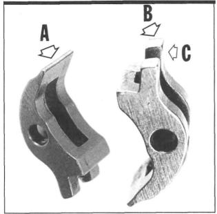
Figure 119- Shows a close view of both sides of the sear and the three inspection areas: at "A", the sear engagement face is checked for damage from battering or alteration, at "B", check for sear/disconnector cycling drag marks or earlier modification, and at "C" check for disconnector drag marking. Replace any questionable sear.
