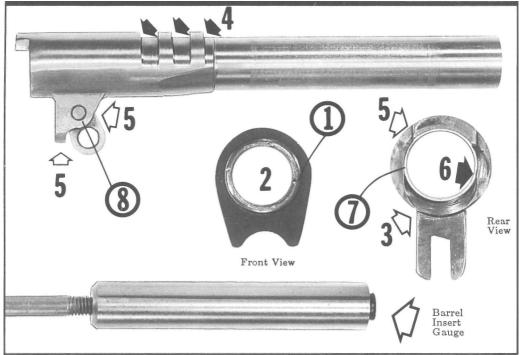
Figure 62- Shows barrel inspection points and, also, a standard service diameter insert gauge, or plug gauge, used to check bores for internal irregularities. Unlike times past, .45 barrels are now in very abundant supply. So, it's foolish to "make dp" by using a barrel in anything less than excellent condition. The present availability of barrels makes welding, remachining, and etc. unnecessary.
