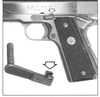
Figure 11- Shows the slide stop lever and half round, milled relief slot in the slide. This slot allows removal of the slide stop by providing clearance for the retaining tip on the back side of the stop. The relief slot in the slide must be aligned with the raised tip of the slide stop retainer before the stop can be drawn out.
