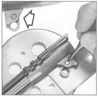
**Figure 69-** Shows increasing lug engagement by re-linking the barrel to a next longer link size. Replacement links are regularly available in seven basic lengths, allowing the barrel and lugs to be raised from the first step of +.003" to +.021". It may become necessary, at a point, to adjust the bottom barrel lug. [See long link.]
