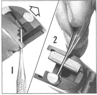
**Figure 21-** Shows a small punch being used with protective pads to withdraw a poorly fit or damaged extractor from the body of the slide. In worst cases, position 1 provides better starting leverage. Position 2 picks up from position 1 and is also useful by itself for removing excessively tight extractors.
