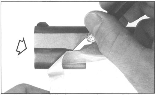
**Figure 213-** Shows detail trimming excess masking tape applied to the prepolished sides of the slide. Use sharp blades and a cutting angle that prevents marking the slide. After sandblasting, the sides are final polished with sandcloth or a felt covered block and polishing compound. This produces the desired finish and also a sharp corner edge where the sandblast begins.
