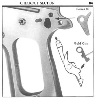
Figure 129- Illustration shows a preassembled sear and disconnector as they would position in the frame. Installation is done with the frame left side up so that small parts such as the Series 80 trigger bar lever can be installed beneath the sear. Preposition the Gold Cup sear depressor and spring; retain with a short pin.
