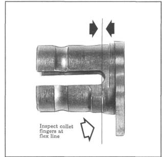
Figure 53- Shows a close view of a collet type barrel bushing, capable of increased accuracy over standard production bushings. Collets have a tendency to break fingers in certain slides, always along the flex line shown above. All the facts aren't yet in, but it seems breakage is related to collet finger O.D. versus slide I.D.
