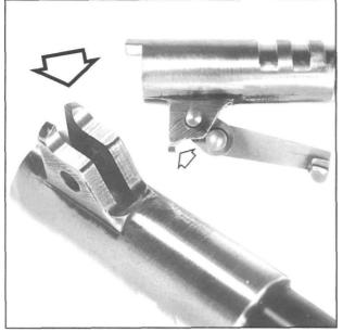
Figure 180- Shows the bottom lug surfaces after having been cut with a lug cutter. When hand fitting is done, the longer link and new, higher lug surfaces, maintain positive vertical locking position. Final lug surface level determines link length. With the barrel fully locked, the lugs should rest on the top and back of the crosspin.
