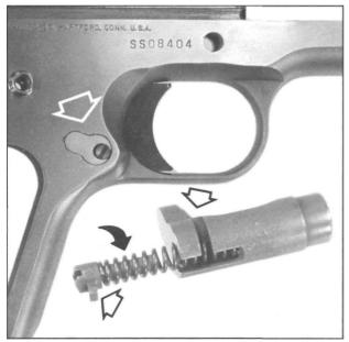
Figure 116- Shows the magazine catch assembly and inspection points. The catch lock [looks like a screw head] is turned clockwise as shown to re-engage its' locking stud in the frame. With the stud positioned inside the engagement recess in the frame, the catch assembly body is then free to retain or disengage the magazine.
