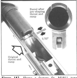
Figure 182- Shows a factory fit, M1911 type barrel positioned on its' frame. Note that the of the barrel and the beginning of the bottom of the barrel and the beginning of the frame ramp. The frame ramp angle is original and unaltered. This untouched state is the ideal beginning point for ramping and throating.
