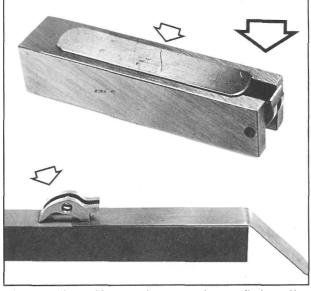
**Figure 125-** Shows the sear in a fitting jig. Angle is adjusted by set screw in the fixture. Hardened spacers placed on top of the jig provide different stoning heights. With this jig, a .040" spacer is used for standard sear length, and a .030 or .020" for tuned. Below, a 45 degree bevel is stoned on the inside sear edge.
