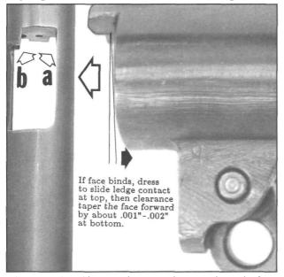
Figure 71- Shows the usual rear barrel face dressing angle. In the fully locked position, the barrel face should be parallel with the slides' ledges. And, it is this position that determines the final face angle. When the barrel has been linked higher, or when battering is found, the rear face angle is usually not correct.
