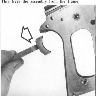
Figure 35- Shows the trigger being removed from the frame. With the body of the magazine catch no longer in place, the trigger and trigger bow assembly are free to slide in their recesses milled inside the frame. This assembly should slide easily out, yet be fit well enough so that vertical movement is minimal.
