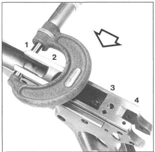
**Figure 162-** Shows parallel checking the outside surfaces of the newly lowered and shaped rails in preparation for slide tightening. To prevent frame caused contact sticking, the rails must be checked at each of the four points shown, and surface polished to within .001" of parallel before the slide is horizontally tightened.
