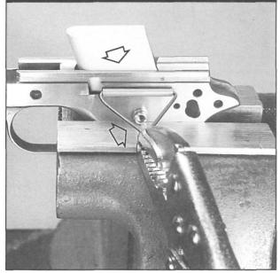
Figure 107- Shows the frame set up in the vise between soft jaw pads, and ready for removal of the plunger tube housing. A magazine well insert prevents bending or distortion of the frame as pressure is applied. Vise grip style pliers and .075-.080" hanger wire are shown being used to draw the housing off the frame.
