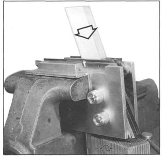
Figure 156- Shows the frame in the vise, set-up between aluminum frame plates, ready for rail peening or swaging. A reinforcing insert, or filler, is. used in the magazine well to prevent frame distortion when the vise is tightened. I suggest using a small lead or wood block under the frame to hold it in vertical position.
