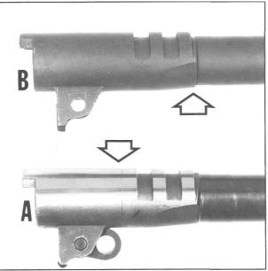
Figure 16- Shows two different examples of M1911 type sleeved block, or two piece, barrel construction. "A" is a typical example of the half lug type sleeve, and "B" is a sample of the more common full lug variation. This easier method of barrel construction economically resolved a number of manufacturing problems.
