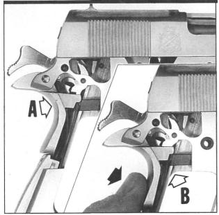
Figure 136- Shows the grip safety in cutaway view temporarily installed for testing. In position "A", the safety is undepressed and the stop surface is long enough to prevent trigger bow movement and sear release. "B" shows the grip safety squeezed and in the bypass position, allowing full movement of the trigger bow.
