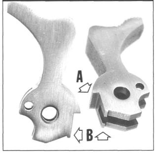
Figure 121- Shows the two inspection points on Series 80 Govt. Model hammers. "A" shows the follow-through stop ledge- no longer captive as with Series 70's and earlier production. Ledge height runs about .075". Keep the ledge in its' original condition. Do not undersize. Full-cock engagement at "B" averages about .030" deep.
