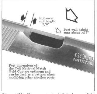
**Figure 189-** Shows a standard Colt factory Gold Cup ejection port. This slide is made with a lower and longer port, and a roll-over clearance notch. Port wall height runs just at .475", and handles almost any ejected shell swing angle. The clearance notch, begins at the forward edge of the barrel hood slot and extends back 3/8".
