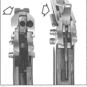
Figure 105- Shows checking ejector/slide and ejector/hammer clearances, after replacement of the ejector. Frame tunnel position and ejector dimensions can vary somewhat, making final clearance adjustments necessary. Installation is not complete until all slide and hammer contact has been eliminated.
