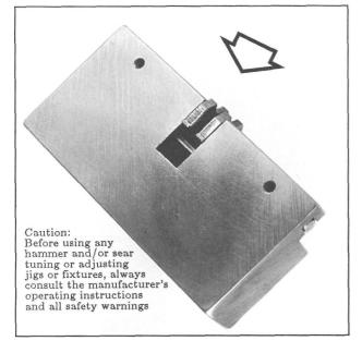
Figure 124- Shows hammer set up in a fitting jig for surface adjustment. Keep the hammers hooks at 90 degrees to the jig top. Position the hammer so the bottom will finish just at the required hook engagement height. If .030" is needed, set the pre-dressed hooks at .030", then work the surface down until just flush with jig.
