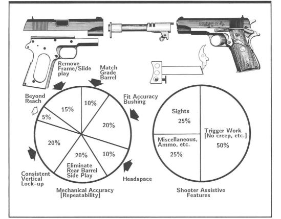
Figure 147- Shows the various elements that produce mechanical, and shooter assistive accuracy in the basic M1911 design. Although this is an over simplification, mechanical accuracy is nothing more than precision fitting and reduction of tolerances until consistent and repeatable function has been reached. Or, in other words, the pistol is tuned, mechanically, to do the same exact thing again and again.
