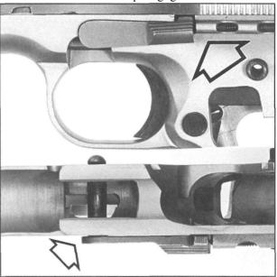
Figure 90- Shows checking slide stop fit in the frame and where to check slide stop clearance. To prevent excess drag and the main cause of false lock-back, make sure the top of the stop clears the bottom of the slide by .015" to .020" [magazine out]. Radius the top locking corner to eliminate catching at the disassembly notch.
