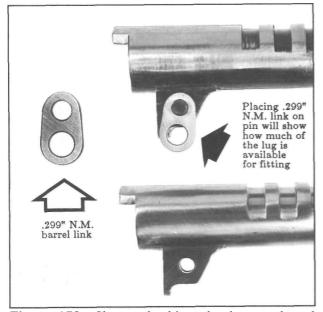
Figure 178- Shows checking the bottom barrel lugs against the longest N.M. link before lug cutting. The lugs must have more than enough bottom material for this link when lugs are cut on a National Match frame. After lug cutting, the new surfaces will be properly contoured, but .002"-.006" over, depending on the cutter.
