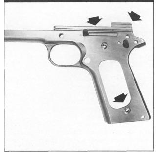
Figure 36- Shows the frame fully stripped, except for the ejector stud, plunger tube, and stock screw bushings. Unless replacing one of these, or detail polishing the sides of the frame, there is no need to remove these items. Now in preparation for inspection, the frame should be thoroughly cleaned with solvent and brushes.
