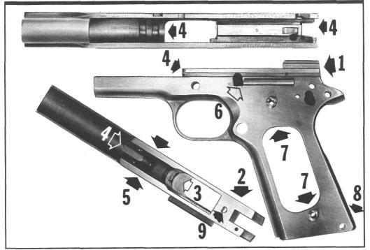
Figure 39- Shows the frame completely cleaned and ready for close inspection and detailing before reassembly. Carefully inspect the areas listed below and detail as necessary. Rusty, bent, damaged, and otherwise substandard frames will not produce a high quality end product, and should not be used.
