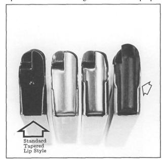
Figure 205- Shows four typical release timing zones and cartridge control lip shapes. If lips are tapered, degree of taper determines release point. With parallel lips, distance apart, and release point position and shape, regulate final cartridge release. Release should coincide with cartridge break-over and extractor pick-up.
