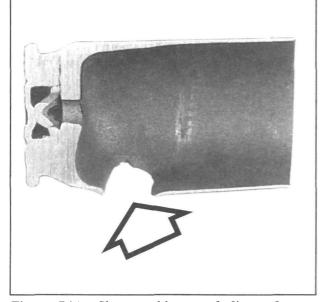
Figure 74A- Shows a blown soft [import] case. The soft brass wall has drawn back toward the pressure vent. The metal insert built into the shooter's Pachmayr grips saved his hand when the magazine blew out. Somehow, the remaining cartridges didn't explode. Primary cause was headspace- secondary cause was over-ramping.
