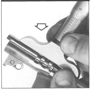
Figure 177- Shows approximating vertical lug engagement using a depth micrometer. Strips of modeling clay pressed into the lugs show slide lug impressions. The micrometer bridge is held at the center line of the lugs, and also toward the light, as the gauge rod is lowered to contact with the upper surface of the clay.
