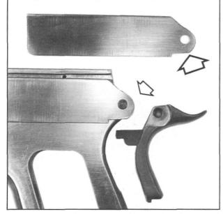
Figure 199- Shows an easily made sheetmetal template used for marking the outline of the revised frame tail. Below, a spare hammer pin is inserted through the hole in the template and then into the safety pivot hole in the frame. This locates the scribe line for the beavertail grip safety. Cut to the outside of the line.
