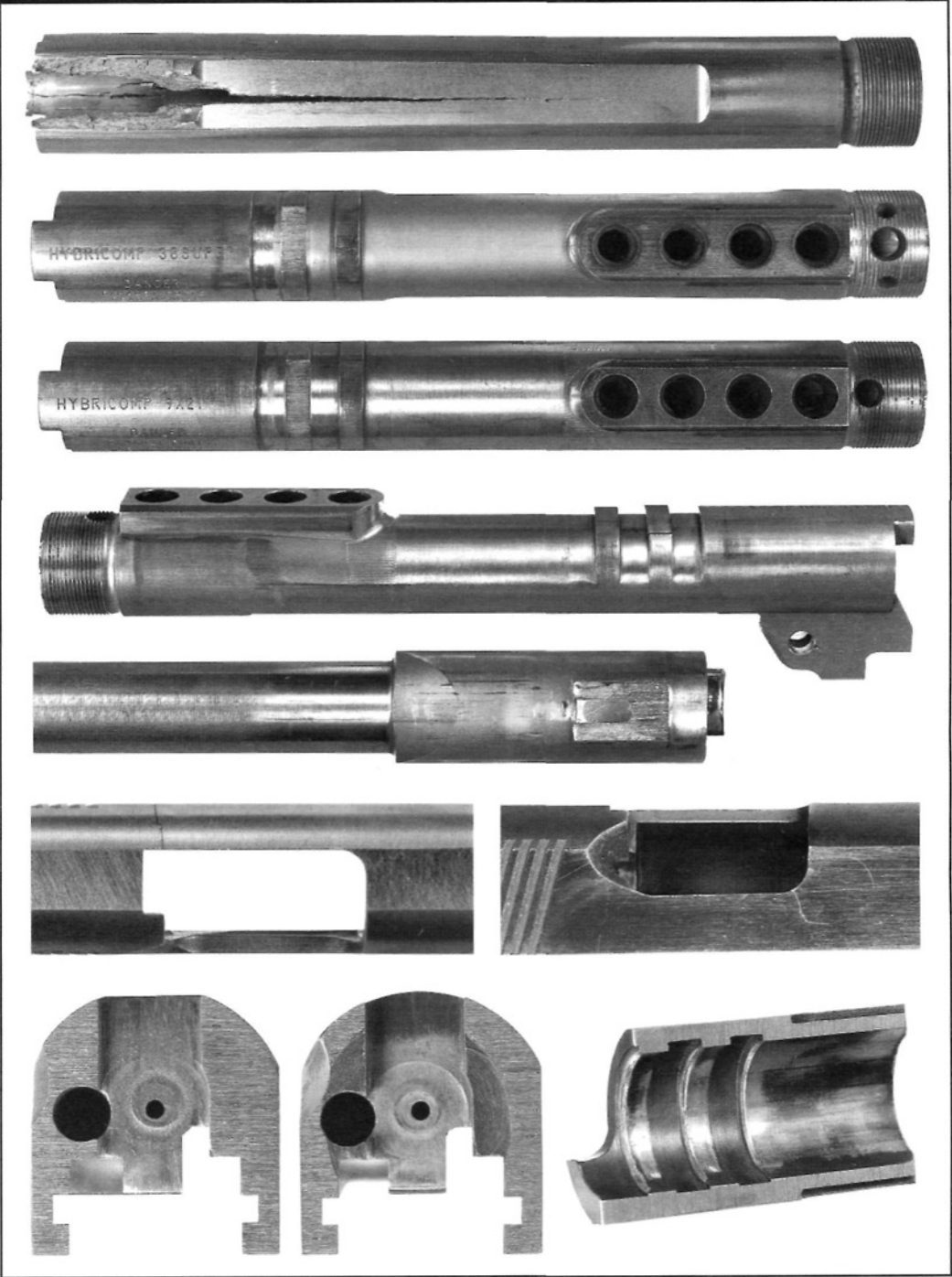
Figure 172- Shows examples of abused custom M1911 components. The barrel, at top, was subjected to an extreme overload. The next three barrels have broken/cracked middle lugs. This damage occurred for two reasons: (1) in all three, only the middle lug was bearing; and (2) a shear force created by 3X design pressure was exerted upon the one bearing lug. The bottom lug sheared off the 5th barrel because of insufficient lower barrel/slide clearance (the barrel could not fully link down). Exterior stress cracks shown in both slides, below, originate at/near square inside corner cuts. Both breech faces show evidence of pressure abuse and firing pin port mislocation in the cutaway sides, at bottom. Barrel lug engagement surface corners are battered/rounded-off in the slide section at bottom right. This damage occurred in a high vertical stack, long barrel link pistol with insufficient slide/top barrel lug clearance at linkdown.
