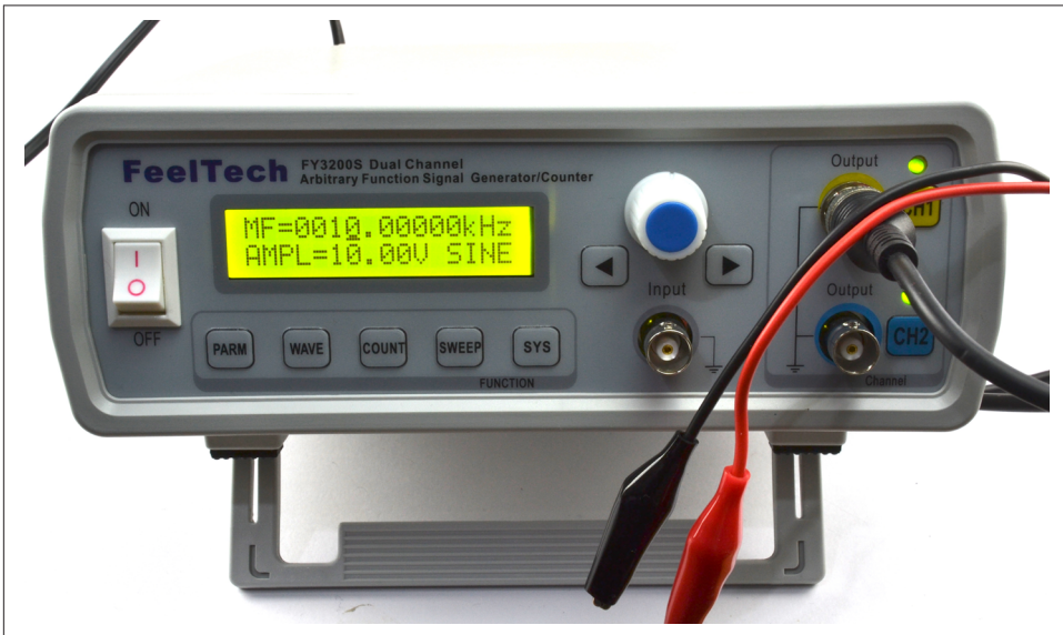
Figure 21-9. A Low-cost DDS (Direct Digital Synthesis) Function Generator
