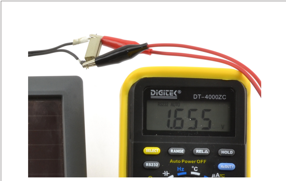
Figure 9-3. Measuring the Voltage Across a Load Resistor
