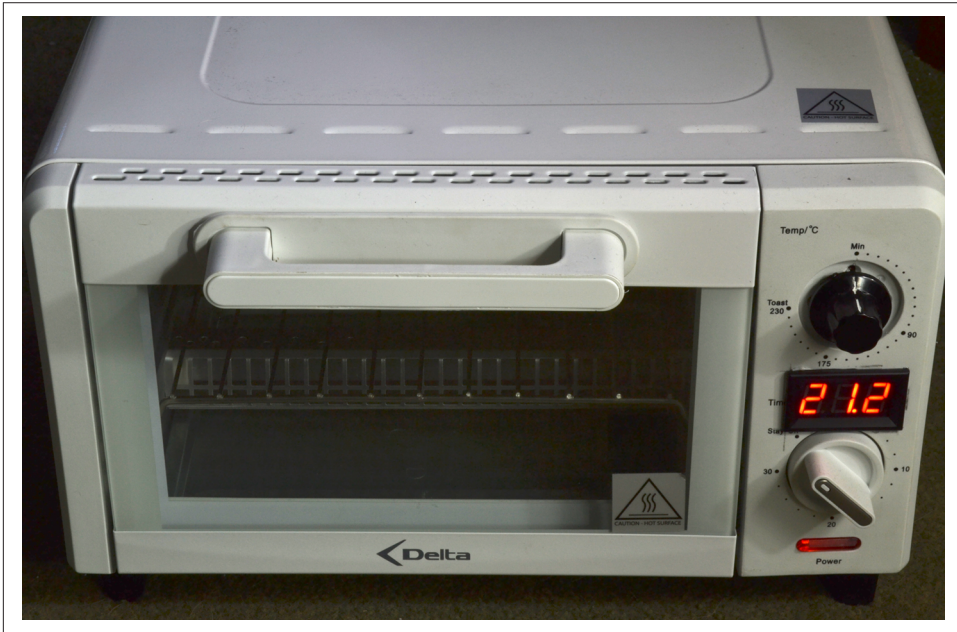
Figure 20-21. A Homemade Reflow Oven
