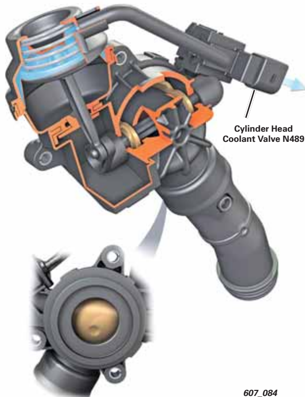
Switching valve closed
