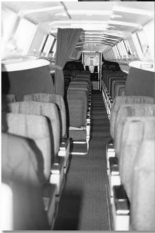
Figure 36. This picture gives a good representation of the interior size of the DC-9. This DC-9 was configured with sixteen first-class seats and eighty-four coach seats. The ONA DC-9 had 105 seats and no first-class section.
