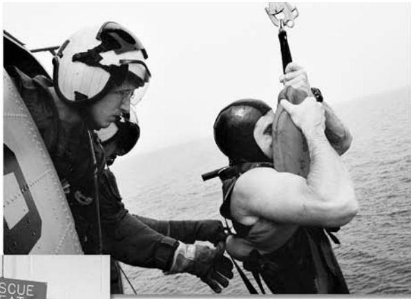
Figure 31. The rescue sling (also known as a horse collar) was one of three methods used to hoist survivors into helicopters. This image shows the correct way to use the sling. Most people stuck their head and arms in first with the hoist cable behind them. Fortunately, the helicopters were low enough that no one fell out.
