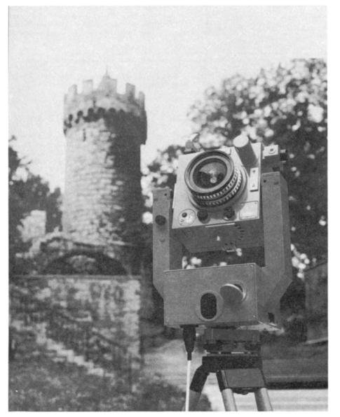
Figure 7.9 Zeiss (Jena) UMK 10/1318 close-range camera
