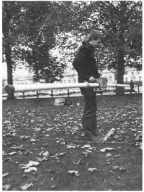
Figure 11.5 Location of gravel-filled channel under St James's Park, London, using ground radar (electro-magnetic profiling) equipment. (*Courtesy*: Wimpey Laboratories Ltd)
