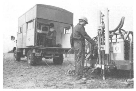
Figure 11.6 Self-boring pressuremeter in operation complete with on-site data acquisition and monitoring system. (*Courtesy*: Soil Mechanics Ltd)
