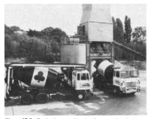
Figure 37.5 Truck mixers awaiting loading at ready-mixed concrete depot. *Note:* conveyor-belt attachment on the truck mixer to the left. (*Courtesy:* British Ready Mixed Concrete Association)
