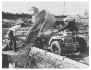
Figure 37.7 1-t turntable dumper capable of depositing concrete over arc of 180°. (*Courtesy*: Benford Ltd)
