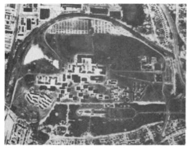
Figure 7.22 Thermal infra-red linescan image of the University of Surrey. (*Courtesy*: Clyde Surveys Ltd)
