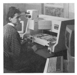
Figure 7.16 Officine Galileo Digicart analytical stereoplotter. (*Courtesy*: Officine Galileo)
