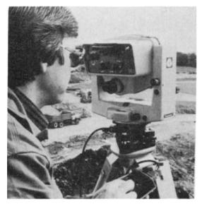
Figure 6.15 Electronic tacheometer, integrated design: Geodimeter 140
