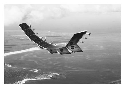
FIGURE 2.1. Helios prototype flying wing, powered by photovoltaic cells, during its record-setting flight above the Hawaiian Islands on July 14, 2001. NASA photo ED 01-0209-6.
