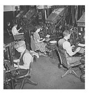
FIGURE 5.3. Mergenthaler's 1890 Simplex linotype design (reproduced from *Scientific American*, August 9, 1890) and composing room of the *New York Times* full of linotype machines (this photograph was taken in 1942 by Marjory Collins).
