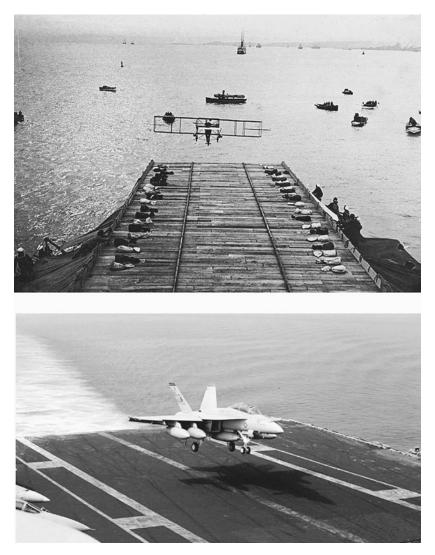
FIGURE 6.8. Development of an idea. Top: Eugene Ely's Curtiss biplane nears the landing platform on the USS *Pennsylvania*, anchored in San Francisco Bay, on January 18, 1911. Arresting lines were fastened to sand bags positioned along the deck. Photograph NH 77608 available at http://www.history.navy.mil/photos/images/h82000/h82737.jpg. Bottom: An F/A-18F Super Hornet nears landing aboard USS *Nimitz* in the Persian Gulf. U.S. Navy photo (030331-N-9228K-008.jpg) by Michael S. Kelly.
