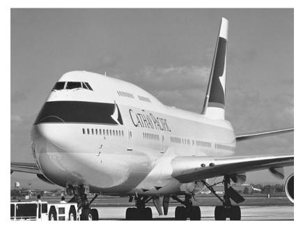
FIGURE 4.13. The Boeing 747, the largest passenger aircraft of the late 20th century whose construction requires more than 100 t of aluminum alloys. Photo from author's collection.
