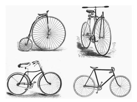
FIGURE 3.17. Evolution of bicycles from a dangerous vertical fork of 1879 and Starley's 1880 Rover (wheels are still of unequal size) to modern-looking "safety" models of 1890s with diamond frame of tubular steel and pneumatic tires. Images reproduced from *Scientific American*, April 19, 1892, and July 25, 1896.
